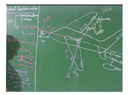
So any motion that cuts this vertical plane of symmetry is known corresponds to a lateral direction corresponds to this lateral directional motion. So what are all the possible cases? Translation along y axis. So this aircraft has to cut this plane of symmetry say let this blackboard be the vertical so this board be the vertical plane of symmetry.
