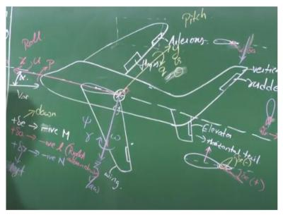
So we have an aircraft. So let us define an axis with respect to which all the components of this aircrafts are mounted. Let us say this as fuselage reference line, right. So we will use this fuselage reference line while talking about stability of an aircraft here. So now let us consider a body access system. So we have wing yeah, let us quickly go through this major components of this aircraft.
