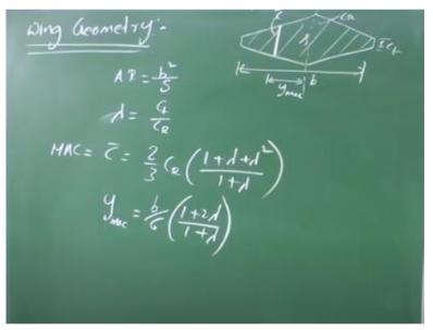
So what we discussed about is the wing geometry. So we talked about some of this non-dimensional parameters. So and so we talked about aspect ratio and taper ratio C t upon C R and then mean aerodynamic chord C bar which is MAC, mean aerodynamic chord is equals to two third upon C R times 1 plus lambda plus lambda square upon 1 plus lambda.
