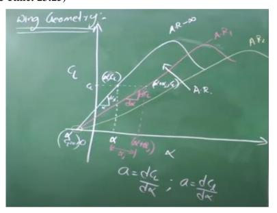
So let us say C L, it is 3D, 3D C L is equals to so sorry is varying with angle of attack here. So let us say this is for an airfoil okay. So this is for an airfoil. This is how C L is varying with angle of attack. So let us assume alpha at with C L is equal to 0, right. Again coming back to this concept when there is no lift that means the pressure distribution on the top and the pressure distribution on the bottom has to be same.
