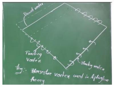
So now, according to this lifting line theory, this wing is replaced say this is the wing that we are talking about, right. So this according to this lifting line theory, this wing is replaced by or the lifting characteristics of this wing is replaced by a vortex sheet, right the horseshoe vortex, right. Now, the part of this vortex sheet which is on the surface of the wing is known as bound vortex.
