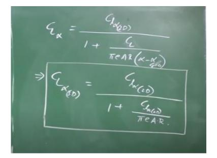
So according to lifting line theory what is alpha i? Yeah, this is C L right, I can write as this C L upon pi e A.R times alpha minus alpha i right. So alpha minus alpha at which C L is equals to 0. Am I correct or not? So what is this C L again? This C L with aerofoil, I will be able to generate by using this expression C l alpha times alpha minus alpha at which C L is equals to 0.
