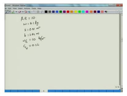
Let us take aspect ratio 10 let take a let us take the data corresponding data, so the wing loading is otherwise the weight of the UAV is 8.1 kg S of the UAV is what? For aspect ratio 10 S is approximately 0.81 meter square. So S is 0.81 because meter square now this is for sorry wing loading of 10 not aspect ratio of 10. I am sorry this is wing loading of 10 so the wing loading so it is simply W upon W by S its 0.81 meter square.
