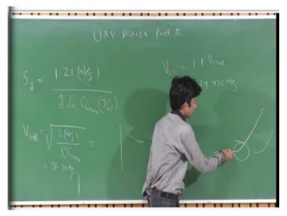
So, let us say your aircraft roll distance is defined by S g, this whole distance means your wheel is at the ground only, ok. This is nothing but 1.2 W by S g rho infinity C L max T by W thrust to weight ratio and this is W by S is a swing loading, ok. So, W by S we have already found out C L max with slight deflection we know ok. And we have to put the value of S g and we have to find out the value of T by W.
