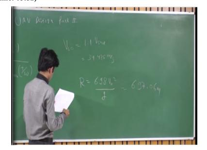
So, in order to pull up your aircraft in takeoff phase, your turn radius will be 6.98 V stall square by g, you just put the stall velocity you will get 697.06 meters pull up radius ok.
