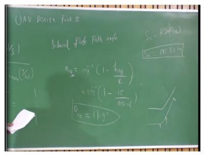
Now we will calculate the induced flight path angle, what should be our flight path during that takeoff? Very important. So, from geometry you will get theta tail theta cos inverse 1 - h OB Justin Pierce notation by R. So, basic a simple geometry, see when you are taking off first thing you have to consider that is screening height in a for certification of any aircraft there is a rule like DCCA or like aircraft rule there is a lot of aircraft rule is there, if you design an aircraft.
