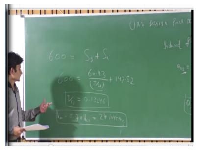
So, total takeoff distance is 600 meters, right, and what is takeoff distance? Is nothing but the ground roll + airborne distance, ok. So, I have given one formula to you S g = 1.21 W by S 0 infinity C L max T by W, if you put W S g which is nothing but 9.81, rho is 1.225, C L max is 2, you will get the relation between S g and T by W which is turned out to be 60.43 divided by T by W + 143.82 and this is 600.
