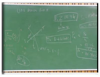
So, your thrust direction will be this and your drive direction will be opposite and your lift will be perpendicular to the free steam velocity, ok. And your weight will act at the downward direction and this angle is nothing but this from this flight path angle you are flying, ok, so this also become the gamma, ok. So, this component will be W cos gamma, right, and sine component will come here, W sine gamma, ok.
