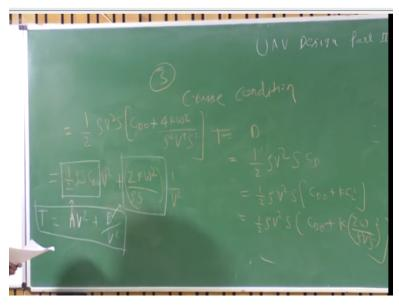
So our third phase is cruise condition, this type of cruise a steady state on level flight, ok, thrust is nothing but drag, drag you can write half rho V square S into C D, half rho V square S C D further you can write C D 0 + k C L square, right, ok. C L what you can write? 2W divided by rho V square S from left you are going to write right. You just put C L value here, what you will get? Half rho V square S C D 0 + k 2W rho V square S whole square, ok, this thing you will get now.
