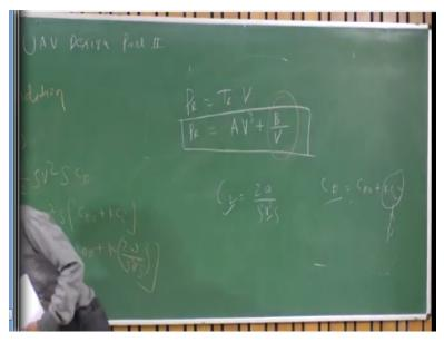
So, now power will be thrust required into velocity this T is nothing but the thrust required. So, if you multiply by V you will get AV cube + B by V this is your power requirement, ok. So, the observation can be made here, as soon as you increase your flight velocity, your this part will go down and this part will rise up. So, this is nothing but the induced drag, this part is induced drag, this is profile drag.
