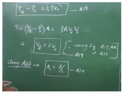
So using these two equations what we have is, subtracting these two this a equation from a from equation from equation b right. So what I have is PR - PL is equals to half rho V 2 square. Let us say this is my equation 18, A18. Now comparing this equation 18 and then previous 15 and 16 what we can write is the thrust generated here or so T is equals to P left minus P or say P right minus P left, right.
