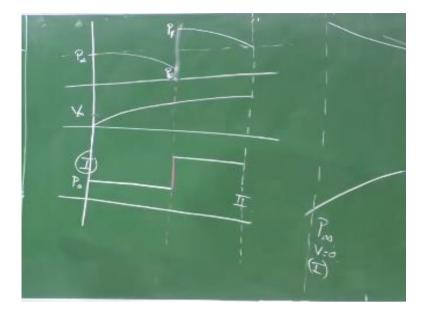
So now okay now let us look at so what we know is about the pressure here right. So let us see how the pressure is varying here. So if this is the location of the disc, right. So what is happening initially say this is my static pressure or P infinity, which is atmospheric pressure. So it drops as we go close to this disc, is it not? Let us say this is the location of this disc, right.
