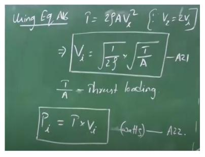
So from this 15 and 16 again using, so using equation 16, using equation A16 what I have is T is equals to 2 rho AV i square, right. Since V 2 is 2V i. So this implies, so the corresponding induced velocity depends upon root over T by A, right. So this particular factor T by A is known as thrust loading. So what is the amount of force generated across this particular area, area of this disc, right?
