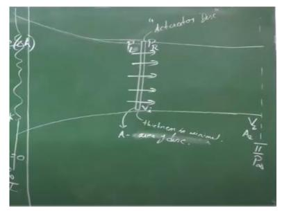
Let us assume this is one such disc called an actuator disc. Let us say this is called actuator disc. So this is called actuator disc, which is capable of creating pressure difference. Let us say this is the upper surface or let us say to the right, pressure to the left, left and this is pressure on the right side. If I take this is my left and this is my right. So I will label them as pressure on left and right.
