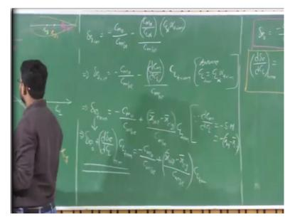
So, delta e trim is equals to minus of C m 0 upon C m delta e, ok, minus of this C m alpha upon CL alpha of the entire aircraft times CL alpha times alpha trim upon C m delta, ok. So, delta e trim = - C m 0 upon C m delta e times d C m upon d CL, right. So, C m alpha upon CL alpha is d C m upon d CL, right, so multiplied by let us assume the total trim angle of attack is dominated by CL alpha times alpha trim, ok.
