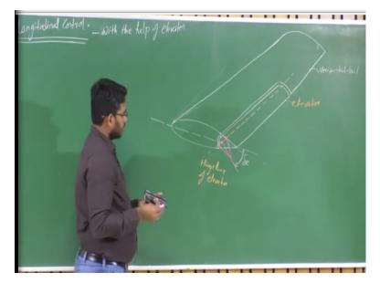
So, let us see what is that what we are going to talk about is longitudinal control, ok. So, how we achieve longitudinal control with the help of elevator? So, let us get back to these equations again, so when I have to increase the velocity what does it mean? I need to produce the thrust which should be greater than the drag at that particular velocity, is not it or not. So, say the engine is producing thrust D which is equals to drag that is nothing but half rho V square S C D.
