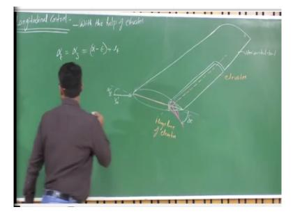
So, as we mentioned this is my chord line, right, so let me draw it a bit clearer. So, say this is my chord line which in the earlier case is the line joining leading edge and the trailing edge, right. And which is nothing but the mean as well, is not it, for a symmetric aerofoil this is nothing but the mean camber line. Now when there is a deflection, what is happening? this chord line is up to this portion is fine is same but there is a change in the mean camber line at here.
