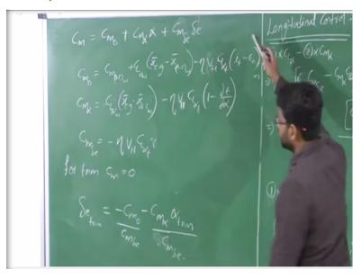
The C m equation which is C m 0 + C m alpha into alpha + C m delta e times delta e, right. So, what should be the control surface deflection to trim this particular aircraft delta e trim? So, in this the C m 0 again see we have wing and we have a tail combination and in the tail we have a elevator right now, ok. So, this C m 0 will still remains the same like C m 0 is equals to C m ac of wing + CL 0 of wing times X bar Cg - X bar ac of wing - eta S t upon S.
