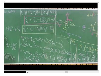
So, this is C L 0 + C L alpha into alpha of the entire aircraft is equals to C L 0 of wing plus C L alpha of wing multiplied by x bar Cg - sorry into alpha wing + eta, this is nothing but alpha, alpha of wing is nothing but alpha here is not it. So, eta of horizontal tail times S t upon S times C L of tail multiplied by alpha of tail, what is alpha of tail 1 - dou epsilon by dou alpha right, alpha into alpha + i of t - epsilon 0 okay.
