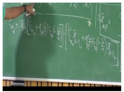
Now so this C m alpha is equals to. So, take out the Cg terms here x bar Cg right x bar Cg times C L alpha of wing okay. So, this is minus into minus becomes plus, + eta of horizontal tail S t upon S multiplied by C L alpha of tail okay. And then the correction factor, 1 - 2 dou epsilon by dou alpha right. So, I am just separating Cg terms in the options here. So, this will be like, okay. So, I have the Cg multiplied by C L alpha is here.
