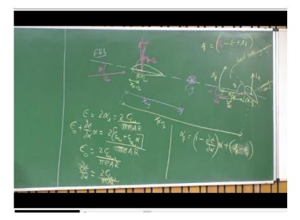
Say the chord of the wing coincides with the fuselage reference line here. So, this is the chord, the chord of the wing coincides with a fuselage reference line. And then we have a tail at after wing right and then we try and also let us not consider about the z offset of the Cg okay. So, we have fuselage reference line and for the wing, we know there is an aerodynamic center for this wing which is located at a distance x ac at the leading edge of the wing.
