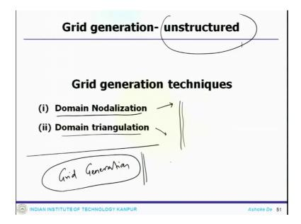
Now the same scenario, gets change when you go down to unstructured grid, here unstructured grid as we have seen throughout this lecture series what kind of element it requires. So, one very common approach is that use domain nodalization approach; that means, you pick a node then calculate the distance and there is a algorithm which is associate with that or you can do a some triangulation kite of approach.
