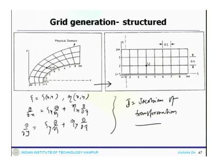
And how you do that? You have this kind of a physical domain and this is what it transform to computational domain and the weight is done, it is essentially goes to a uniform xi eta direction and as it can be xi x y and eta this would be x y.
