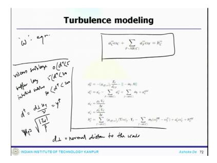
So, this will return all the term one can think about the omega equation 2, so all these equations will appear there. Now one important thing it will happen is that calculation of the wall function. Because all this turbulent equations these are having used and that time and the thing is that near the wall flow field resolution is very important, if you have a domination of the viscosity.
