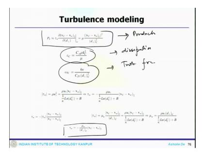
Similarly, this is the turbulence production term and this is the dissipation term which can be estimate at that cell. And, this is the turbulent frequency term and one can estimate the wall shear stress also.
