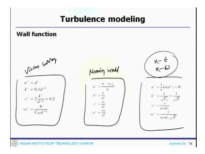
Now, if you go to, so sublayer, then this is how u plus and y plus they are connected and if you have a moving wall, then u plus is connected like that viscous sublayer and for k and epsilon typically this is what done k or omega. So, for 2 equation models this is how it is done.
