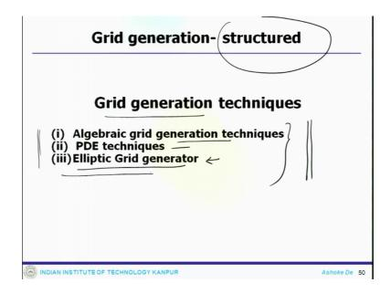
Now, typical gird generations technique if it is a structured system, then either one can use some kind of a algebraic grid generation technique which can take care of this different calculations algebraically and then generate the gird or can solve for the PDE techniques. PDE means you solve for the partial differential equation and then get the well or elliptical gird generator; that means, you solve for some elliptical PDEs.
