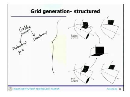
Now, grid generation if you recall you can actually all your realistic complex grid would be in this nature. When you have a complex grid this kind of a nature either you have option of generating unstructured grid, that is one option or you can generate a structure grid; structure grid then you need to transform this kind of system to xi eta system or the regular coordinate system.
