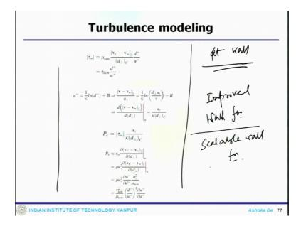
So, one you estimate all these I mean these are the calculation for that and one can actually get all this calculation for at wall this information can be calculated. Now, the other way one can think about using some sort of an improved wall function because what happens that sometimes the grid resolution is not sufficient.
