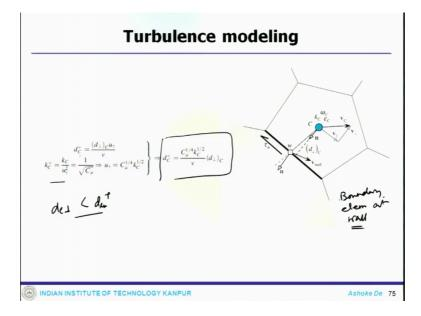
Now, one can see when it comes down to a boundary element this is a boundary element and I mean where close to the wall and you have to boundary element at wall because the normal calculation needs to be done. So, one can calculate the normal distance d c plus
