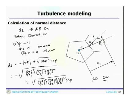
Let us see a 2 dimensional control volume or 2 dimensional control volume, how do you calculate the normal distance? So, the normal distance can be calculated is just using some sort of an based on solving a differential equation. So, this can be calculate by solving a differential equation and which could be solving a like and Poisson, Eikonel or Hamilton Jacobi kind of equation.
