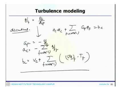
So, and if you solve the turbulent flow problem and use everything in the in your in your governing equations, you get this geometric diffusion coefficient; geometric diffusion coefficients at the face is E f by d cF. And your discretized equation would get modified like a c phi c plus face n b c a F phi f is equals to b c, here a F equals to minus g f which we got here then a c equals to minus summation over f g f and b c equals to V c plus f which is del phi f dot T f.
