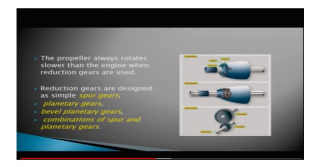
The propeller always rotates, slower than the engine, when the reduction gears are used so, with the help of reduction gears, the propeller RPM is reduced, reduction gears are designed as simple spur gears, planetary gears, bevel planetary gears and combination of spur and planetary gears. So, there are various types of reduction gears, they may be spur gears, bevel glares, bevel planetary gears, planetary gears or a combination of spur and planetary gears.
