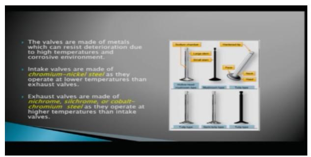
The valves are made of metals which can resist deterioration due to high temperature and corrosive environment, now the valves, these valves are also exposed to very high temperatures and corrosive environments, so they need to be made of metals which can resist deterioration due to this high temperature and corrosive environment.
