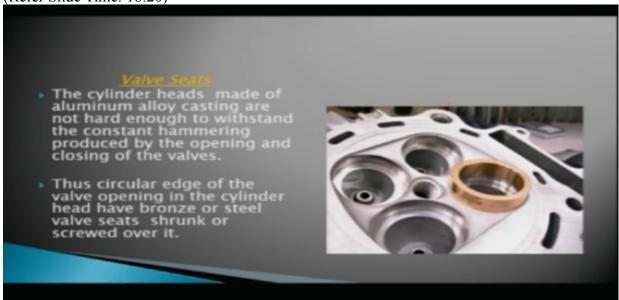
Next is valve seats, the cylinder heads made of aluminum alloy casting are not hard enough to withstand the constant hammering produced by the opening and closing of the valves, so when the valves are continuously opening and closing they're providing the hammering on the cylinder head and cylinder head being made of cast aluminum alloy, they are not very strong, they are not very hard enough to withstand this hammering, so in order to avoid that valve seats are provided on the valve openings.
