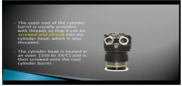
the outer and of the cylinder barrel is usually provided with threads, so that it can be screwed and shrunk into the cylinder head which is also threaded, so this is your cylinder barrel area,
