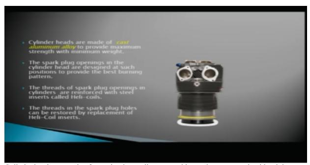
Cylinder heads are made of cast aluminum alloy to provide maximum strength with minimum weight, so cylinder heads they are cast, they are made of cast aluminum alloy so that your weight is kept to minimum and it also has maximum strength.
