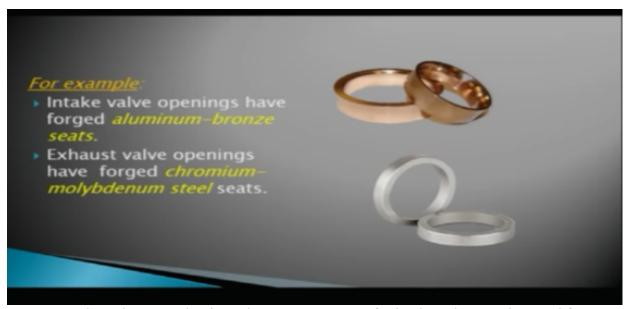
you can see here these are aluminum bronze seats meant for intake valve openings and for exhaust valve openings you have chromium molybdenum steel seats.
