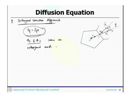
Then one can do second way of doing that that is called orthogonal correction approach. So, what you do here again you get this particular two elements, they are connected as usual and the component of the surface vector one would be along this line, if this is theta and the other one would be along this line the perpendicular one ok.
