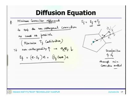
So, let us start with let us have this cell connected which is let us look at this picture. So, this is a approach called minimum correction approach. So, this is for the decomposition of S f through minimum correction method or approach.
