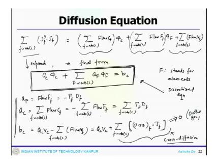
Now if you take it slightly more or expand it slightly more so, what we are having at the left hand side is the flux going for all the faces and after decomposition or expanding we get now summation over all the faces it is flux C f phi c plus summation over all the faces flux F f phi f ok. And so, this you can put it in the bracket plus summation of f going over c you have flux v f.
