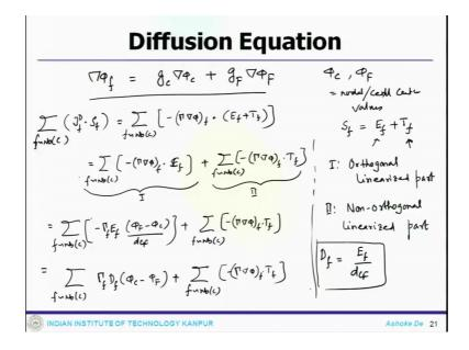
Now what one can do the gradient at the face can have two contribution; one at g c delta phi c plus g F delta phi F where phi c phi, F are the nodal or cell centre values. So, you use the information of the cell centre values to get this particular information.
