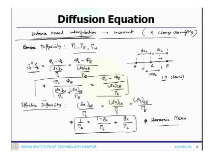
This is a distance based interpolation, it can have problem or rather it can be incorrect in some particular cases like that where or rather one can say that these distance based interpolation can lead to some sort of an incorrect results, when there is a sudden or abrupt change in conductivity. If kappa changes abruptly then this kind of distance based interpolation will have a problem.
