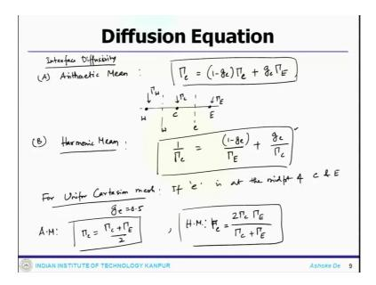
So, the interface diffusivity for interface diffusivity there are two option simpler option A, one can use some Arithmetic mean arithmetic mean expression which is essentially writing like gamma e equals to 1 minus g e gamma c plus g e gamma E where your elements are sitting C E west. So, this is the interface of e this is the interface of w and this guy will have gamma E, this guy will have gamma C, this guy will have gamma W.
