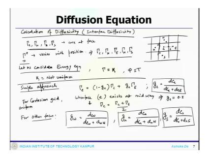
So, in our equation system or the discretized equation system, we have written these diffusive coefficients like gamma e, gamma w, gamma s, gamma n, gamma s, like that. So, these are actually the coefficients that belong to faces.
