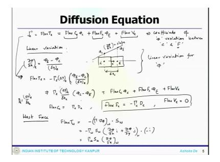
And once we get the discretize system, we assumed a this is a linear variation for phi between points C e or west. So, once we have done the linear variation, that slope will give that profile of that. From there, we have calculated each of these coefficients for the total flux definition with the linear variation. And once we obtain that, and we have defined one more parameter that D capital D for each faces these are defined as E W west, north and the definition lies here.
