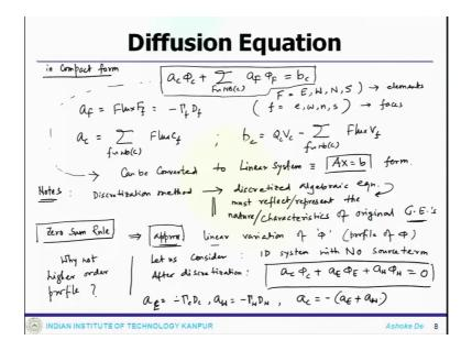
So, in compact form if you write that will look like an a C phi C plus summation of f which will go from all the faces a F phi F equals to V c. And what a F stands for? A F stands for flux F f which is minus gamma f D f ok. So, where small f is east, west, north, south that is how they a C is summation of small f goes from this flux c f and b c that would be Q c V c minus summation of small f flux V f.
