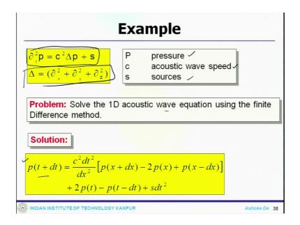
Now, the example that we have taken that if you look at it that wave equation; that solve the 1D acoustic wave equation using some. The governing equations is this where delta is the Laplacian, p stands for pressure, c is the wave speed, s is source and solution would be of this nature, p t plus delta t and x plus dx and all these. (Refer Slide Time: 24:18)
