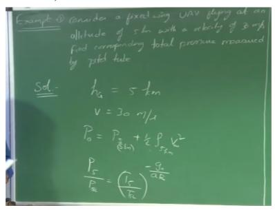
First example is consider a fixed wing UAV flying at an altitude of 5 kilometers with a velocity of 30 meters per second. Find corresponding total pressure measured by the pitot tube? So the information that is given here is geometric altitude is 5 kilometers, so first we need to find the total pressure measured by the pitot tube. So we have velocity of the flight vehicle as 30 meters per second.
