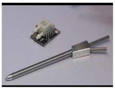
Let us look at this pitot-static tube, see the holes that you can see on this periphery are meant for static pressure and you can see one hole which is along the longitudinal axis of this tube that is meant for total pressure right. So these holes are along the circumference of this outer tube right. You can consider there are two coaxial tubes, one with the closed mouth, the other with the open mouth here right.
