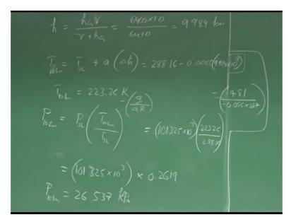
Now first we need to convert hG to h for this hGr/r+hG, this=6400/6410 which is 9.984 kilometers right. Now the corresponding temperature at that altitude is why because if I want to know what is the static pressure at 10 kilometers, in the previous example we witnessed we need to find temperature at that particular altitude right. So T at 5 kilometers from the definition of lapse rate is T at sea level, 10 kilometers is T at sea level+lapse rate times delta h.
