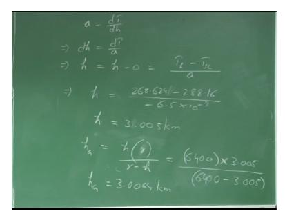
Now I know what is the temperature at this particular altitude h right by using definition of lapse rate, a=dT/dh and what we need is dh=dT/a, dh is h because with reference to sea level I can write dh as h here, h2-h1=h-0 that is=T at altitude-T at sea level/a. This implies h=268.624-288.16 is the sea level temperature/-6.5\*10 power -3 Kelvin per meter.
