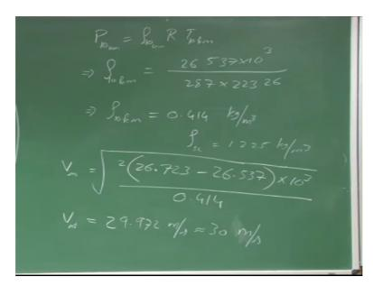
So by using the equation of state, P at 10 kilometers=rho at 10 kilometers R\*T at 10 kilometers. What we have here is density at 10 kilometers is=what is P at 10 kilometers is 26.537\*10 power 3/287\*223.26 Kelvin. So this implies density at 10 kilometers is 0.414 kg per meter cube. So density at sea level is 1.225 kg per meter cube right, 1.225 kg per meter cube. See the density is decreased by more than half.
