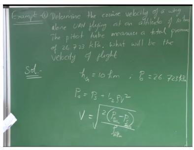
Determine the cruise velocity of a wing alone UAV flying at an altitude of 10 kilometers. The pitot tube measures a total pressure of 26.723 kilopascals. What will be the velocity of flight? So we need to determine the velocity of flight at 10 kilometers altitude. So hG is 10 kilometers and what we have is total pressure at 10 kilometers altitude is 26.723 kilopascal right, kilopascal okay.
