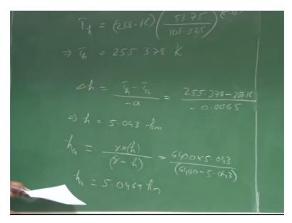
So the temperature at this altitude is=288.16 Kelvin times temperature pressure at that altitude 53.75/101.325, so both are in kilopascal 1/5.25 right. So this=temperature at that altitude is=so 255.378 kilopascals sorry Kelvin. So you have the temperature, now by using the definition of lapse rate delta, h=T2-T1 or Th-T at sea level/-a this=255.378-288.16/-0.0065.
