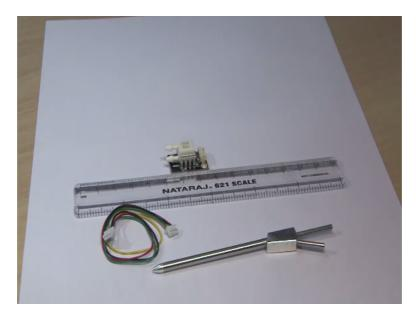
There is a differential pressure sensor, you can see the scale of this sensor is about a centimeter long right less than a centimeter and the total sensor size is about 2 centimeters right. This is the differential pressure sensor and the size of this sensor is about 2 centimeters here including the PCB which helps you to acquire the data right and it weighs hardly 15 grams right.
