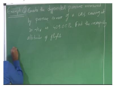
Consider the differential pressure measured by the pressure sensor of a UAV cruising at 30 meters per second is 0.4 kilopascals. Find the corresponding altitude of flight?
