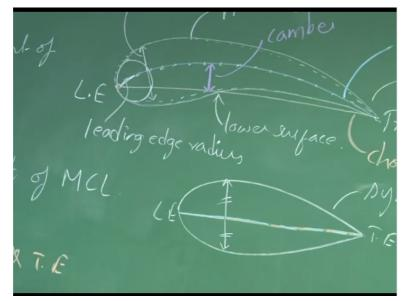
So this curvature which is tangent to the upper and lower surface right is known as leading edge. If you draw a circle with a radius such that the circle becomes tangent to the upper and lower surface alright. So that radius is known as leading edge radius. We call this as leading edge radius okay. Now how can I plot this airfoil? When I say plot here, I need the coordinates of upper and lower surface. How can I plot it? Or say how an airfoil often works?
