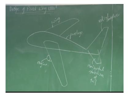
So let us assume this as an aircraft right. So you have so the major components are wing, horizontal stabilizer or tail, vertical stabilizer or vertical tail right and we have a propulsion system that is engine, here it will be on either side right. You can have a single engine as well in some of the aircrafts. So you have fuselage and then undercarriage right.
