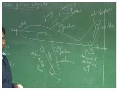
And you have flaps or high lift devices which are used to enhance the lift right. We saw that lift is essential, we nomenclature just now a force that opposes the weight right. So lift so if you want to enhance the lift at a lower velocities, we need to operate this flaps right and you have flaps at the same time you also have spoilers which can sometime be used as a control surface as well, you also have spoilers.
