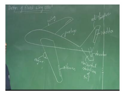
So hence these moving components are also known as control surfaces. Some of these moving components are known as control surfaces right. So we have something on elevator as well as so we have something on horizontal tail called elevator, it is a moving surface right which helps to control the nose up and nose down motion right and there is a moving component on this vertical tail called rudder which helps you to turn left and right.
