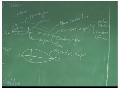
Now comes the camber, the distance between this mean camber line and chord line is known as camber, mean camber line and chord line right okay got it. Now say if the camber is 0 what happens? What is camber 0? When the mean camber line coincides with this chord line, so in that case the thickness distribution will be symmetric about chord line.
