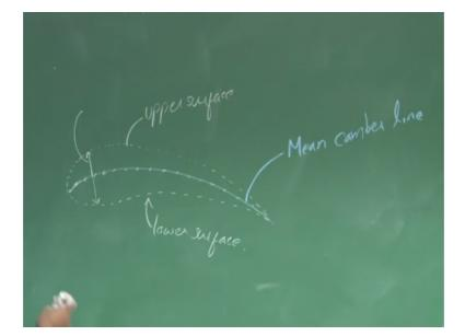
So let us consider an arc or a line like this alright. Let us say this is let us nomenclature it as Mean camber line. What is this mean camber line right? Now if I want to draw an airfoil with the help of this mean camber line what should I do? I can build the entire airfoil with the help of this mean camber line right. So let us say I know the thickness distribution at each and every point right.
