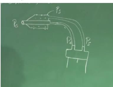
Instead of measuring pressure separately from pitot tube and static tube what you can do is you can connect to a differential pressure sensor right. One can be P0, the other can be Ps. So you can have a pitot tube, you can connect pitot tube to this total pressure port and then you can have a static tube at the same time. So we will get Ps from here, P0 from here right. So
