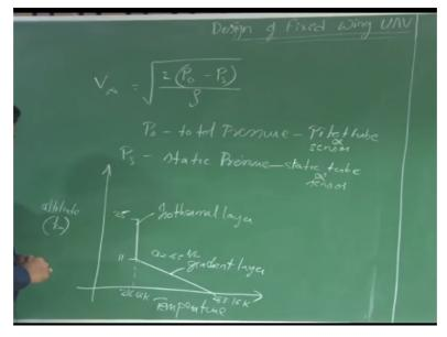
So we derived that if you know the differential pressure that is if you can measure the total pressure, static pressure and if you know the density you will be able to find the velocity. So we measure this total pressure right with the help of pitot tube and static pressure with the help of static tube and corresponding pressure sensor, static tube right connected to a pressure sensor, static pressure measured with the help of static tube connected to sensor pressure sensor.
