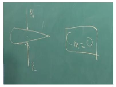
And also suppose this is the symmetrical airfoil your net upper pressure and lower pressure acting let us say PL and net upper pressure acting is PV so this will act at the same point. So, there will be the no lift and no movement so in this case CM=0 okay. And for the tenth question fur positively tempered airfoil produces in bracket it is also given moving is positive. So, you know that for the tempered airfoil the CMAC is negative.
