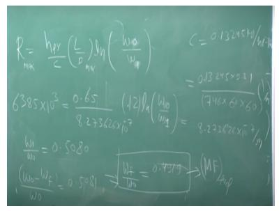
Using this formula R = eta p r/c c is the break excess fuel consumption which is given 0.13245hp kg per hp alright this is kg/hp hour okay. So, you can use this formula L/D ln w0/w1, w0 is the weight when all the fuel gets consumed and w1 is the initial weight. This is w1 and w0. w0 is the total weight of the air vehicle and W1 is the weight when all fuel gets consumed. So, R max is given, if this is the R maximum this also will be the maximum, okay.
