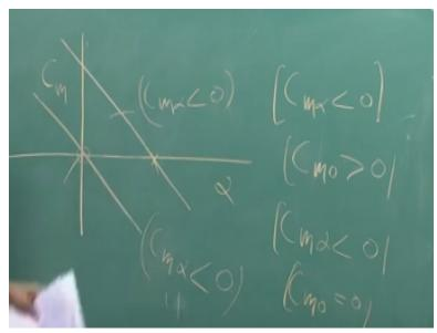
So, as you know that from this diagram you can say in you angle of attack is in x axis and pitching co efficient is y axis. So, this is your CM versus alpha graph for the stable UAV in this condition CM alpha < 0. So, this is the necessary condition in this case CM alpha < 0 but CM0 at
