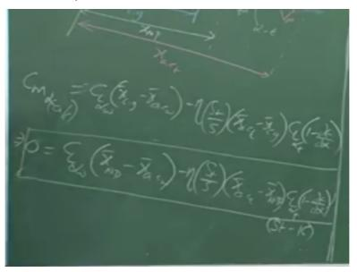
Now, we will address that so, what; so, let us say this is the CM alpha is 0 that means, let us consider this CM alpha of this wing and tail combination here, what is that? CM alpha of the aircraft which means, which implies, CM alpha of the entire aircraft is 0, about this CG location, right, so that particular CG location is known as neutral point, so what is the CM alpha of this wing and tail combination? We derived it just now.
