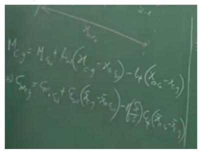
Moment about CG of this aircraft is; moment about aerodynamic centre of the wing + lift of wing, see moreover we have not assumed any offset of this CG with respect to fuselage reference line, so z CG is not considered, so since we are considering, say if this is your; this
