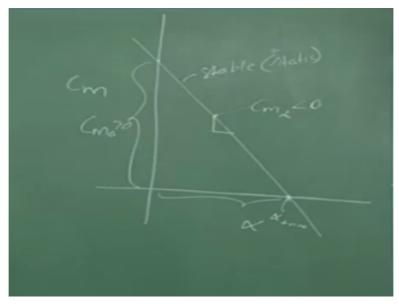
So, we witnessed that the CM with variation of angle of attack for this UAV should have a negative slope, so this is considered as stable system, stable and it is static, staticalistic or static stability, so the negative slope itself does not guarantees that it is statically stable, this CM alpha is < 0, the slope here is < 0, it is the necessary condition but the sufficient condition should be CM0 should be > 0 here, right.
