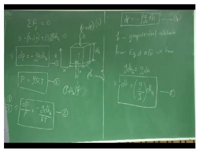
Consider an infinitesimal fluid element with rectangular cross sections, right, rectangular faces in unit cross sectional area. Each face is having unit cross sectional. Let this face be, let us label this as A and the top face be B, right. Say these 2 faces, it has a unit cross sectional area and these 2 faces are separated by distance dh, right. So further since it is a fluid element, there will be forces acting on it, right.
