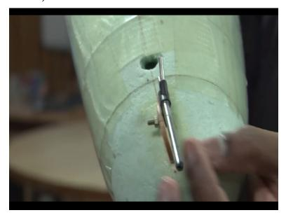
See this is one VTOL UAV which we are right now working on. This was built by our team members and I do not know whether you are able to see this pitot tube or not, but I will try to make it clear, right. So this is your pitot tube and there is a coaxial tube here where you have the holes on the surface with a closed mouth that is your static tube.
