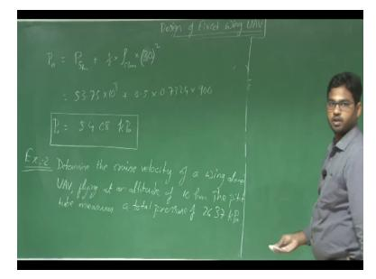
So what do we get, P0=P at 5 km+1/2 rho at 5 km\*, what is V? V infinity square which is, yes, V 30 m/s, right. So what is P at, is 53.75 KPa+0.5\*0.7324\*900. So this is equals 54.08 KPa. So this is the pressure measured by the pitot tube which is installed in this UAV, right, which is flying at 5 km altitude at a speed of 30 m/s. Now take another example. Example 2. Determine the cruise velocity of a wing alone UAV flying at an altitude of 10 km, right.
