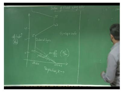
So this typical plot represents how the temperature varies with altitude. It continues, right. So it is up to say 11 km, right. Initially the x axis here is temperature in Kelvin, right. Y axis here is altitude, h or hG you can say, right. So this is in km, okay. So initially it is observed that there is a change with respect, temperature change with respect to altitude. After a while there is a constant temperature regions and again there is a gradient regions, right.
