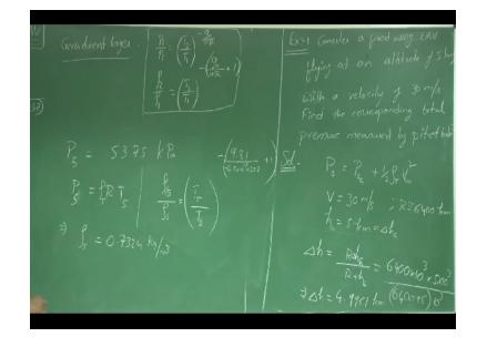
So if you solve this equation, what you get is static pressure at 5 km which is equals to 53.75 KPa and the corresponding density at this altitude is, what you can do is simply by, you know equation of state which is P=rho RT. P at 5 km=rho at 5 km R\*T at 5 km. Now you can directly solve this since you have P5 and T5. Otherwise you can also use this equation like rho 2, rho at 5 km/rho at sea level=T at 5 km/T at sea level, raise to the power of -9.81/-6.5\*10 to power of -3\*287+1, right.
