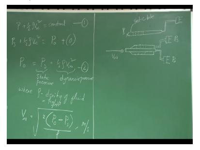
This is with the closed mouth. And again I make a small drill at this end and tap the corresponding pressure by means of this pressure sensor. Fine. Now if I have to capture this static pressure, what I need to do is to drill the holes along the surface or on the circumference of this tube, right. So I can tap static pressure by using this sensor, using this setup. This particular tube that helps you to capture this static pressure is a static tube.
