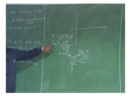
So we know aircraft, aircraft have 6 degrees of freedom here, right. We can translate as well rotate along the three access here of this body frame. So it can translate along xyz and rotate along these three access, so the rotation along the x body x-axis is known as Roll and Pitch and Yaw, right. You have Roll, Pitch and Yaw of the system.
