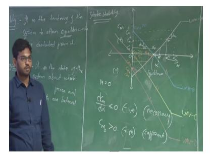
Consider the Cm variation with angle of attack; since we mentioned it is an aerodynamic moment so these aerodynamic force and moment depends upon the angle of attack, right. Let us consider this variation of Cm with angle of attack. So let us say this is for the entire aircraft or a UAV entire UAV. So say in the first case you have a UAV which is, so let us say this is you UAV-A. This is your UAV-B, right. So what is this particular point?
