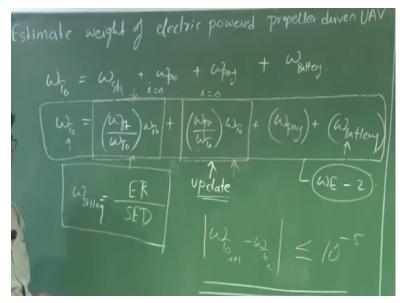
Where the total take of weight us a summation of structural weight, propulsion weight, weight of the propulsion system, weight of the structural system and of course there is a pay load, which is guided by the mission requirement and then what you have is fuel weight or battery weight. We can express this equation in terms of weight ratio and propulsion weight ratio times the total take-off weight and pay load is a given input and value battery need to be estimated as per the requirement, right.
