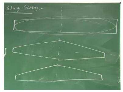
So how you are doing this, wing sizing. So what are the wing parameters in the first place. We discussed about some of the planform parameters, right. You can have a rectangular wing, you can have a tapered wing, tapered about midpoints of the chord, right. Tapered about trailing edge, right or an elliptic wing. So there can be many planforms, right. So what are the major parameters that we need to consider here while sizing the wing.
