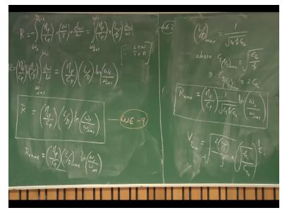
So L/D max=1/root over 4K CD0, right where CL for L/D max is root over CD0/K and CD for L/D max=2 CD0, twice the profile drag, the induce drag=profile drag in this case. So if you substitute this, the range maximum will be eta p/Cp\*1/root over 4KCD0\*ln of Wi/Wi+1, right. This is the maximum range that you can obtain for a given fuel load. And the corresponding velocity for R max will be root over twice the wing loading/rho\*root over K/CD0 to the power of 1/2 or 4th root over CD0, right.
