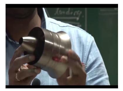
There is also a ducted fan, right which is also powered by electricity like we use onboard battery to power this particular power plant. You can see here there is a fan, right. So the output again here is a shaft power. See this is the back side of this particular EDF. We call it as electric ducted fan. So the output is a shaft power here. It has a similar concept of this outrunner motor, brushless outrunner motor.
