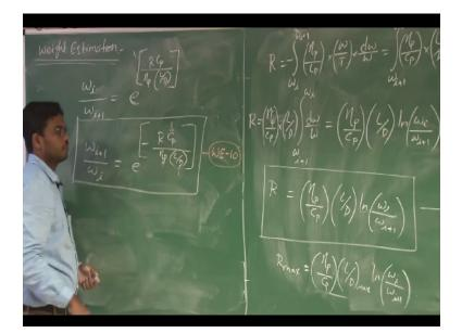
So or say Wi+1/Wi, otherwise Wi/Wi+1 to start with, =e raise to the power of R\*Cp/eta p\*L/D, right. So this is the weight fraction, then Wi+1/Wi=e raise to the power of -range\*Cp/eta p\*L/D. So this is your fuel-weight ratio that you need to carry. This is your WE-10. So if you want to have a range, right, as per your mission requirement, you need to carry this much fuel load.
