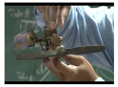
It is a small IC engine, right. So these are carburettors that controls the fuel-air mixture and there is a valve inside with which you can control this fuel-air mixture and the corresponding RPM, right and the shaft power. So what is shaft power here? The power that is available along this shaft, right. So it is in, this is a mechanical power that will be available by, so this is a fuel inlet, the valve that you can see here is a fuel inlet, right.
