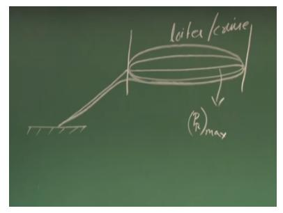
We are trying to perform Engine sizing right so if you look at a typical profile of machine profile of UAV what it has to do is. It has to climb to a particular altitude and then say cruise or say loiter which effectively is a cruise here and then decent to the home right. So, this loiter is performed by cruise right. So, what we have estimated is what should be the minimum and maximum power requirement.
