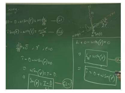
So, when we move this UAV at a particular velocity so we have lift acting perpendicular to it and drag acting along this V infinity right. So, due to weight of this system acts perpendicular to the local horizontal so this flight is moving at an angle gamma with respect to this local horizontal. The corresponding component of weight perpendicular to this V infinity is w cos gamma.
