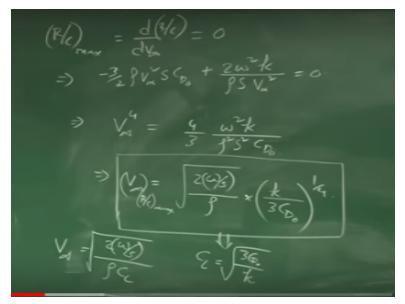
So, rate of climb if I need the maximum rate of climb for this rate of climb max I differentiate this rate of climb with V infinity and equate it to 0 for rate of climb maximum right. So, that implies -3/2 rho V infinity square S\*CD0 and this will be-+ 2w square\*k/rho\*S\*V infinity square=0 alright this implies V infinity to the power of 4=4/3 w square\*k/rho square S square CD 0.
