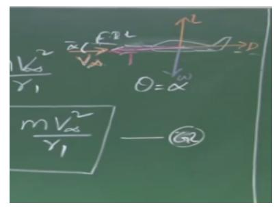
So, this is your reference axis and say this is your thrust, this is your V infinity, this is the reference axis, this is your thrust T and this is your v infinity, the lift acts perpendicular to v
