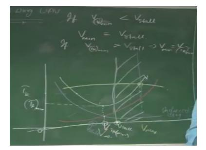
Now, which one we need to consider as the limit; lower limit, there is an ambiguity right, now if V max or V for thrust required minimum that is nothing but the minimum velocity for level flight right, which is = V minimum is < V stall, right, otherwise, this V; velocity for thrust required minimum is < V stall, then minimum velocity during cruise = V stall right. What does it mean? So, we have a stall velocity here right, so this is your stall velocity, V stall in the first case.
