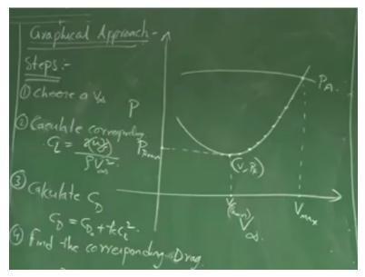
Power with velocity, so for a propeller driven aircraft aircraft, power required varies with the velocity, right, this is how it typically looks like and power available from the power plant almost remains constant, right, so this particular intersection point will help you to figure out what is the corresponding maximum velocity that you can fly during level flight, right and again the minimum velocity that we have already discussed.
