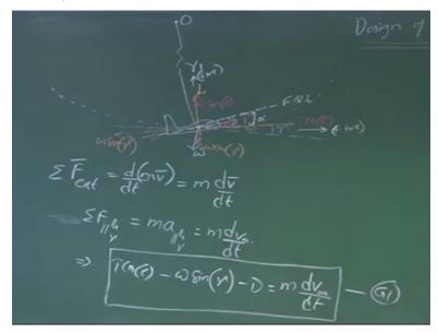
Now, let us go back to the general equations of motion, let us consider this is your UAV acted upon by external forces thrust, due to this thrust, the aircraft; and you have weight acting vertically down and due to this thrust, the aircraft will move at a certain velocity; V infinity, so this is your V infinity and once it start moving, there will be flow due to which there will be lift aerodynamic forces, external forces like lift and drag.
