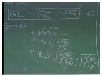
Once I have this L/D max, I can immediately find what is the thrust required minimum condition, right, this = w/; what is L/D max, L/D max which is L/cD max, this = w \* root over 4k cD0, if you know the profile drag of your aircraft of your UAV and if you know what is the induced drag correction factor, you will be able to find out what is the minimum thrust requirement of that system for a given UAV, right of weight, w.
