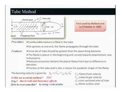
Let us look at a tube method what you can do? Tube it is a horizontal tube which a you feel with the fuel oxidizer mixture to start with and then of course, there is a some kind of nozzle you can say through which the you know mixture can move when the flame front is moving right.
