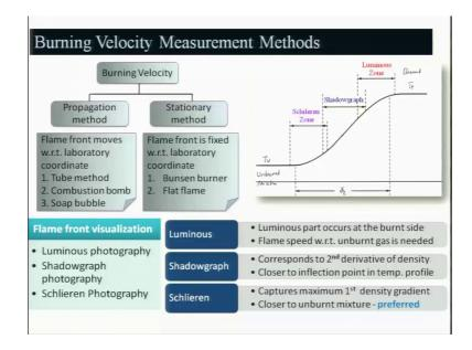
And this measurement methods for burning velocity can be broadly divided two categories one is the propagation method or when the flame will be moving at certain velocities, other is the stationary method like where the flame has to stabilize and then you measure the burning velocity.
