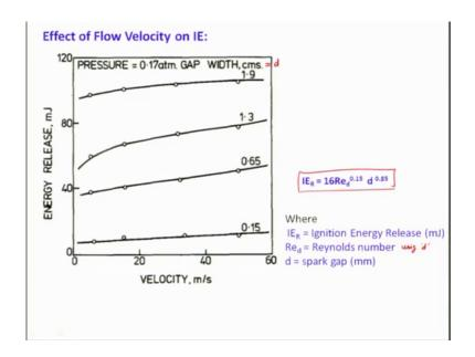
And this is the energy is not really related to minimum energy, it is about the energy which will be released whenever you apply some gap width between the spark electrode and certain pressure you will be giving right.
