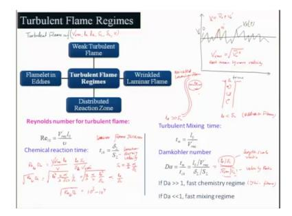
So, this turbulence one will be weak turbulent flame, other is will be wrinkled laminar flame; that means, it will be wrinkling the flame surface, but it is laminar in nature right, and flamelet in Eddies, and distributed reaction zone. Now question arises we have talked about it, but how we are going to basically divided into 4 categories.
