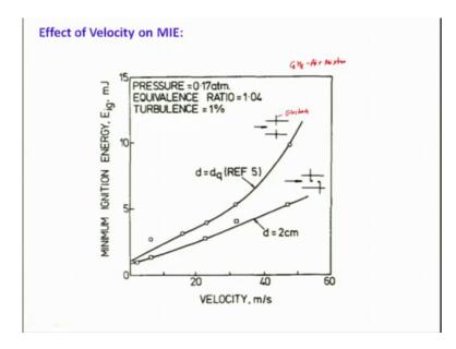
Let us look at the effect of velocity on the minimum ignition energy right. Here the situation is like that turbulence is 1 percent very low turbulence. And equivalence ratio 1.0 and this is basically C 3 H 8 air mixture right. And pressure is 0.1 atmosphere and that depends on the how this electrode these are basically electrode right. And flow is this way like electrode are being arranged it is what type of electrode right. And this is a line itself like a alone if the flow this is different.
