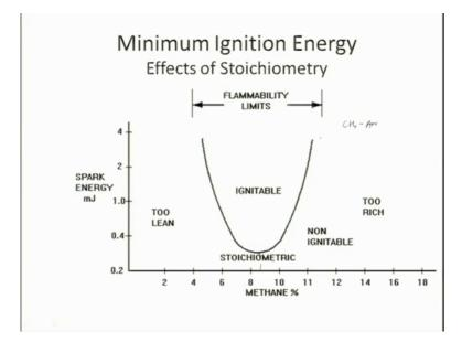
So, if you look at this is the you know data which I have shown spark ignition energy versus methane air percentage of methane air methane. And this is for methane air system C H 4 air flame.
