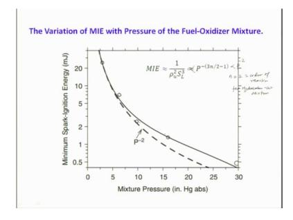
And let us see that variation of minimum energy ignition minimum ignition energy with pressure for fuel oxidizer, we have seen that the minimum ignition energy is proportional to power pressure basically, P power 3 n by 2 minus 1. If I take the order of reaction is something 2 right. This is your order of a reaction right for a hydrocarbon air mixtures if I take certain range right.
