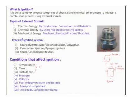
So, if you look at the ignition is a quite complex process comprises of basically physical and chemical phenomena. Like means there will be mixing will which will be occurring. And also there will be the kinetics of the chemical kinetics, the chemical reaction will be taking place to initiate a combustion process using external stimuli.
