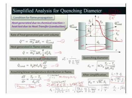
So, now we will be looking at a very simplified analysis to determine the quenching diameter rather we will be relating that laminar burning velocity with the quenching diameter. So, we always talk about a quenching distance kind of thing, where the flame is entering into a tube. These are the wall. So, if you look at this is the wall, right of the tube.
