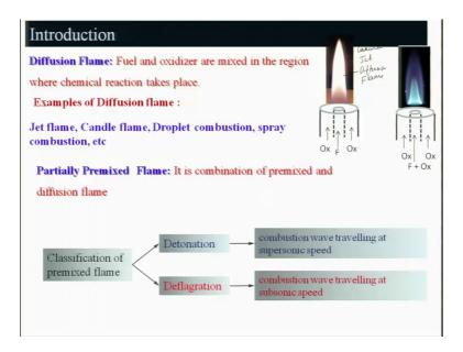
Now, the diffusion in case of diffusion flame the fuel and oxidizer are mixed in the region, where the chemical reaction takes place right. In other words fuel and oxidizer are mixed on the surface of the flame itself right. As I told earlier it is like your marriage I had related that you know fuel and oxidizer basically you can consider one is male and female like you know, and then the marriage will be occurring; that means, you know
