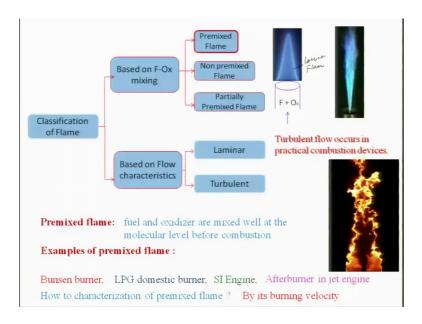
The flame can be you know classified on various basis one is the extent of mixing right the extent of mixing of fuel and oxidizer we can classify, and we can also classify based on what you call the physical state like whether it is a gaseous fuel flame or a liquid flame right or a solid fuel flame kind of things we can do that.
