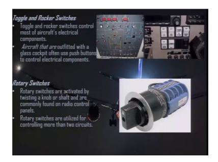
Now, toggle switches and rocker switches in the diagram this diagram you can see these are the toggle switches this is the toggle switch various types of toggle switches, you can see this toggle and these are the rocker arm switches toggle and rocker switches control most of the aircrafts electrical components aircrafts which have glass cockpit are generally using push buttons to control electrical components rotary switches rotary
