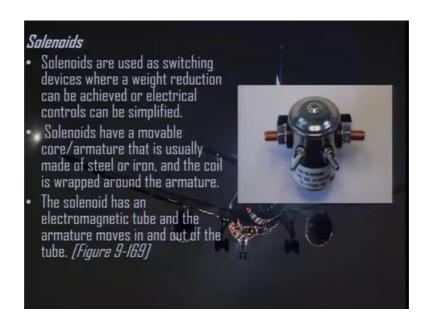
Solenoids are used as switching devices where a weight reduction can be achieved or electrical controls can be simplified solenoids have a moveable core that is usually made of steel or iron and the coil is wrapped around the armature the solenoid has an electromagnetic tube and the armature moves in and out of the tube.
