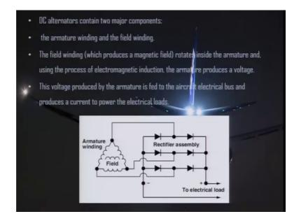
Dc alternators contain two major components the armature winding and the field winding. So, in the figure here you can see there are two types of windings one is the armature winding another is the field winding the field winding which produces a magnetic field rotates inside the armature and using the process of electromagnetic induction the armature produces a voltage.
