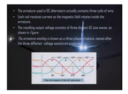
The armature used in DC alternator actually contains 3 coils of wire each coil receives current as the magnetic field rotates inside the armature the resulting output voltage consists of 3 distinct AC sine waves as shown in the figure. So, you can see 3 waves 3 sine waves here the armature winding is known as a 3 phase armature named after the different 3 different voltage waveforms produced.
