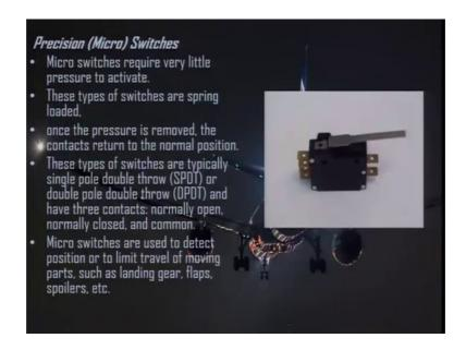
Precision micro switches micro switches require very little pressure to activate these type of switches are spring loaded once the pressure is removed the contacts return to the normal position these types of switches are mainly single pole double throw or double pole double throw and have 3 contacts normally open normally closed and common micro switches are used to detect position or to limit travel of moving parts such as landing gears flaps spoilers etcetera.
