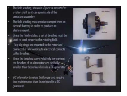
So, this field winding which is mounted on the rotor shaft this spins inside the armature assembly the field winding must receive current from an aircraft battery in order to produce an electromagnet. So, field winding has to receive current from an aircraft battery.
