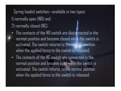
Now, another type of switches spring loaded switches they are available in 2 types normally open we call them a no condition and normally closed nc switch the context of
