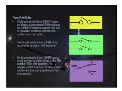
Now, types of switches there are various types of switches single pole single throw switch this opens and closes a single circuit pole indicates the number of separate circuits that can be activated and throw indicates the number of current paths. So, pole indicates the number of separate circuits that can be activated and throw indicates the number of current paths.
