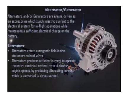
Now, coming to alternator or generator alternators and or generators are engine driven as an accessory which supply electric current to the electrical system for in flight operations while maintaining a sufficient electrical charge on the battery. So, alternators or generators they are in general and they generate electricity and supply electricity for flight operations and also to maintain sufficient electrical charge on the battery.
