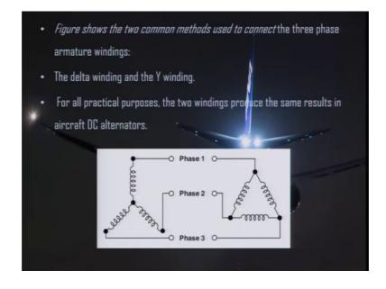
Now, in this figure you can see two common methods which are used to connect the 3 phase armature windings delta winding and the Y winding in both the cases windings produce the same results in a craft DC alternatives.
