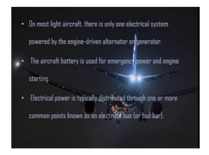
In a single precision engine aircraft electrical system on most light aircraft, there is only one electrical system powered by the engine driven alternator or generator
