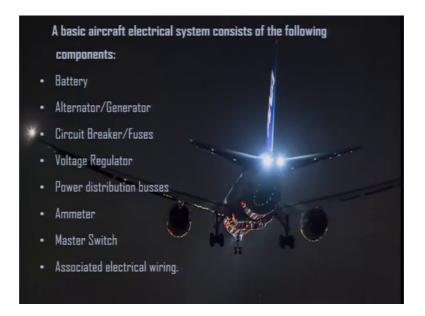
Basic aircraft electrical system consists of the following components. So, some of the basic components in a simple electrical system are battery alternator or generator, circuit breakers, fuses, voltage regulator, power distribution busses, ammeter, master switch and associated electrical wiring. So, these are some of the basic components.
