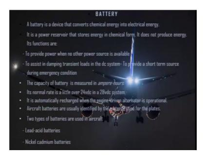
Battery another component very important component in an aircraft electrical system battery it is a device that converts chemical energy into electrical energy; it is a power
