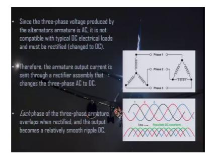
Since the 3 phase produced by the alternator armature is AC it is not compatible with typical DC electrical loads and must be rectified change to DC now the 3 phase voltage which is produced by the alternator armature is AC it has to be converted to DC therefore, the armature output current is sent through a rectifier assembly that changes the 3 phase AC to DC.
