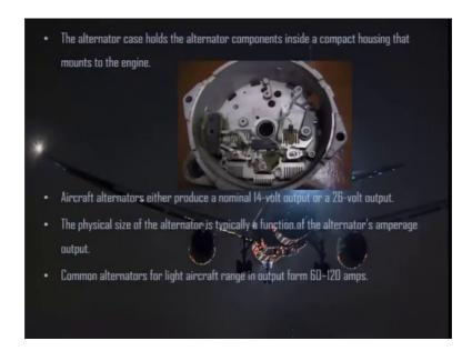
The alternator case you can see this is the alternator case here this is the alternator case this holds the alternator components inside the compact housing that mounts to the engine aircraft alternators either produce a nominal 14 volt output or a 26 volt output the physical size of the alternator is typically a function of the alternators and pure h output common alternators for light aircraft ranges in output from 60 to 120 amperes.
