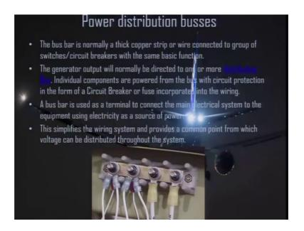
Next is power distribution buses the bus bar is normally a thick copper strip or wire connected to group of switches or circuit breakers with the same basic function the
