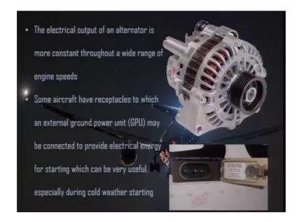
Electrical output of an alternator is more constant throughout a wide range of engine speeds some aircrafts have receptacles to which an external ground power unit may be connected to provide electrical energy for starting which can be very useful especially during cold weather starting.
