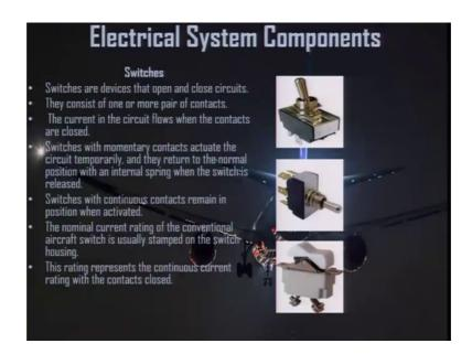
Now, coming to various electrical system components the various electrical system components very important parts switches they are the devices that open and close circuits they consist of one or more pair of contacts the current in the circuit flows when the contacts are closed. So, when the contacts are closed the current will flow in the circuit switches with momentary contacts actuate the circuit temporarily.
