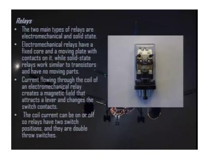
Relays the 2 main types of relays are electromechanical and solid state. So, 2 types of relays are mainly used either electromechanical or solid state electromechanical relays
