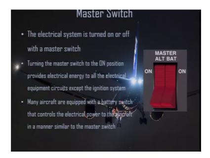
Excess master switch; the electrical system in an aircraft is turned on or off with the master switch this is a very important switch in an aircraft to turn on or off the electrical system master switch is used. So, this master switch is a very very important component of the aircraft electrical system turning the master switch to the on position provides electrical energy to all the electrical equipment circuits except the ignition system.
