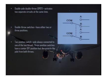
Double pole double throw this will activate 2 separate circuits at the same time. So, this diagram, you can see, this is a double pour double throw switch. This will activate 2 separate circuits at the same time double throw switches have either 2 or 3 positions to position switch pole is always connected to one of the 2 throws 3 position switches have a center of position that disconnects the pole from both throws.
