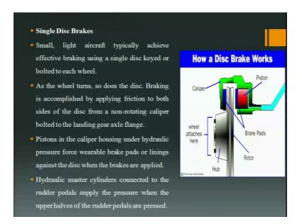
As we are getting better materials now a days the use of carbon discs is increasing in the modern aviation fleet. Now, coming to single disc brakes, so how a disc brake works you can see in the diagram, this is your hub assembly this your wheel, wheel. Now this rotor you can see here rotor, this is the disc which is attached to the wheel hub.
