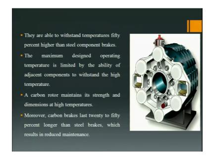
The carbon fiber discs are noticeably thicker than the sintered standard steel rotors, but are extremely light, these carbon brakes they are able to withstand temperatures 50% higher than the steel component brakes.
