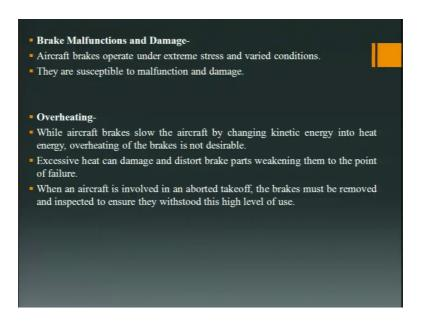
Brake malfunctions and damage, aircraft brakes operate under extreme stress and varied conditions they are susceptible to malfunctions and damage. Overheating; when while aircraft brakes slow the aircraft by changing kinetic energy into heat energy, overheating
