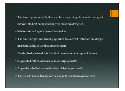
The basic operation of brakes involves converting the kinetic energy of motion into heat energy through the creation of friction. So, basically the kinetic energy is being created is being converted into heat energy through friction, modern aircraft is mainly using disc brakes. The size, weight and landing speed of the aircraft influence the design and complexity of the disc brake system.
