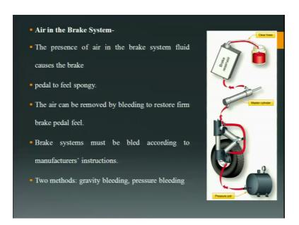
Now, air in the brake system as I just mentioned in case, there is air in the brake system what will happen you will feel that the brakes are spongy, so how to remove air in from
