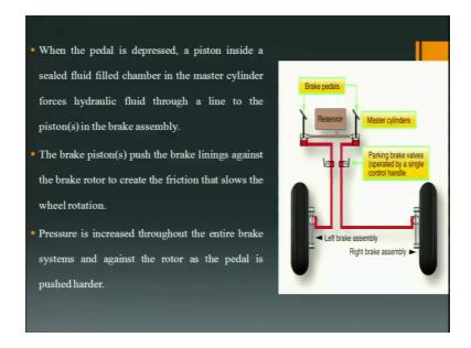
Now, when this pedal is depressed a piston inside a sealed fluid filled chamber in the master cylinder, in this master cylinder there is a piston here, and there is a chamber which is filled with fluid. So, when the pedal is depressed piston inside a sealed fluid filled chamber.
