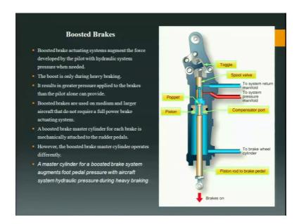
Now, boosted brakes actuating systems augment the force developed by the pilot with hydraulic system pressure when needed. So, as the name suggests this boosts the brake the force developed by the pilot this will boost the force developed by the pilot with hydraulic system pressure when it is required.
