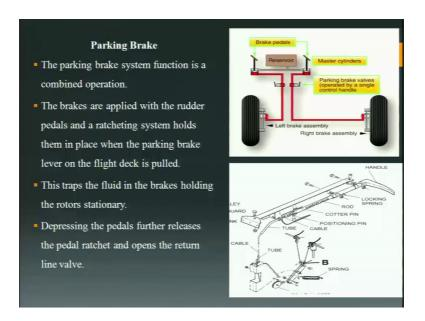
Now, parking brakes, parking brakes they are a very important part of the brake system the parking brake system function is a combined operation. So, this is the diagram for in this stop diagram you can see this is the diagram, where you can see the brake pedals here, these are the reservoirs now master cylinders, in the master cylinders you have the fluid reservoir also this is your brake line.
