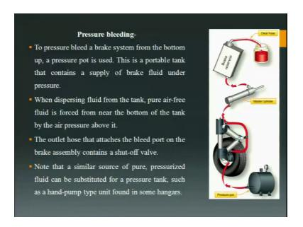
Now, pressure bleeding you can see in the diagram this is the pressure pot here, this is your brake unit this is your brake line this is your master cylinder, from the master cylinder this is the brake reservoir and from the brake reservoir and from the brake reservoir you have a container which has got the hydraulic fluid.
