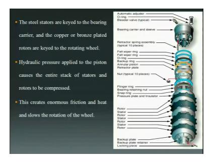
The steel statuses are key to the bearing carrier, these steel statuses they are keyed to the bearing carrier this is your bearing carrier, these stators are key to the bearing carrier and the copper or bronze plated rotors.
