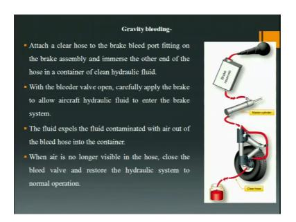
Another method called the gravity bleeding. Same thing you can see here this is your brake reservoir you are pouring in fluid hydraulic fluid in the brake reservoir from the brake reservoir, it is coming to the master cylinder from the master cylinder via the brake linings it is coming to the brake unit at the brake unit there is a bleeder port a hose is attached to the bleeder port and this hose is inside a container having hydraulic fluid.
