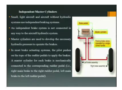
Independent master cylinders, this is basically the independent type of brake actuating system, which has got independent brake master cylinders. In the diagram you can see, these are your rudder pedals, these are your master cylinders, these master cylinders have a reservoir, fluid reservoir. Then these are your brake linings, this is your brake lining this your brake assembly here, and this is your wheel.
