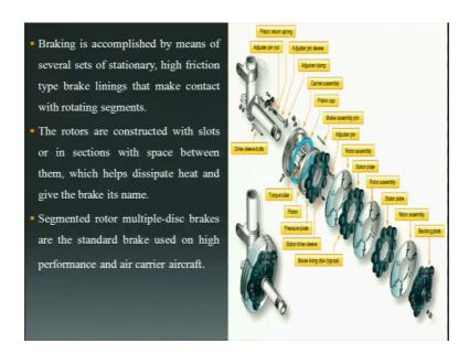
So, they are used with high pressure hydraulic systems or power brake systems, braking is accomplished by means of several sets of stationary, high friction type brake linings that make contact with the rotating segments. So, similarly as in the multiple disc brakes braking is accomplished by means of several sets of stationary, high friction type brake linings that make contact with the rotating segments.
