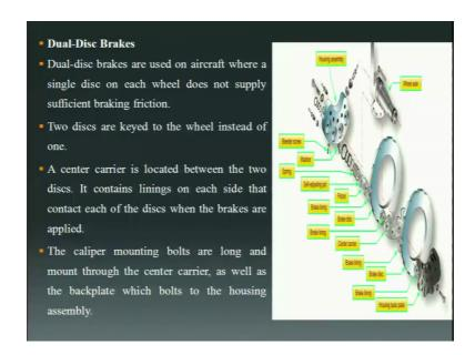
So, as the aircraft sizes became larger, single disc brakes were not effective. So, there was a necessity to have brakes which could provide more braking action. So, dual disc brakes were design, dual disc brakes are used on aircraft where a single disc on each wheel does not supply sufficient braking friction in these dual disc brakes there are two discs you can see in the diagram.
