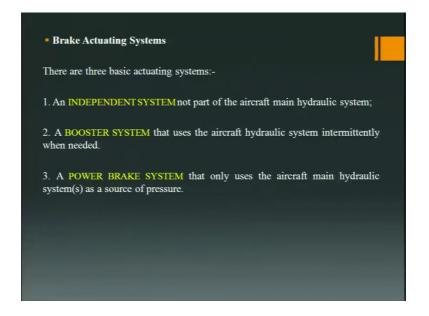
So, the different type of brake actuator systems, there are mainly three types of basic actuated systems one is the independent system, booster system, power brake system. Again depending on the type of brakes, type of aircraft the brake actuating systems are designed the independent system is not part of the aircraft main hydraulic system that is an independent system.
