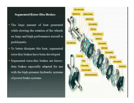
Now, another type of brakes where we have segmented rotors, so the discs they are of discs they are of disc type only, but the discs are segmented the large amount of heat generated while slowing the rotation of the wheels on large and high performance aircraft is problematic and due to friction large amount of heat is generated and this large amount of heat can be of problem.
