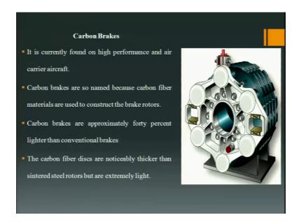
Now, another type of brakes carbon brakes, it is currently found on high performance and air carrier aircrafts carbon brakes are so named, because carbon fiber materials are used to construct the brake rotors. Carbon brakes are approximately 40% lighter, than conventional brakes. The carbon fiber discs are noticeably thicker than sintered steel rotors, but are extremely light.
