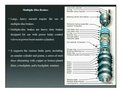
Now, another complex type of brakes is the multiple disc brakes, we have seen the single disc brake, we have seen the dual disc brake. Now this is multiple disc brakes, large heavy aircraft require the use of multiple disc brakes; multiple disc brakes are heavy duty brakes designed for use with power brake control walls or power boost master cylinders. So, as we have mentioned earlier depending on the type of aircraft depending on the size of the aircraft the brakes are designed.
