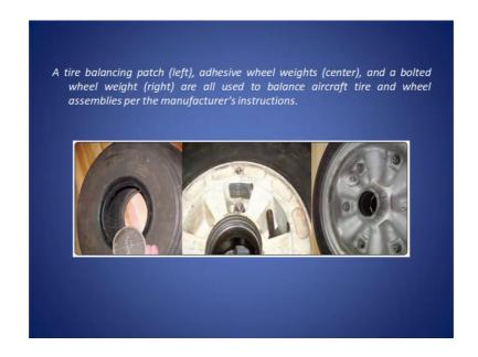
So, here in the diagram you can see a tire balancing patch, this is the tire balancing patch on the left side, these are adhesive wheel weights in the centre and a bolted wheel weight you can see this is the bolted wheel weight on this in this right diagram, they are all used to balance aircraft tire and wheel assemblies, as per the manufacturer's instructions.
