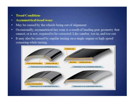
Now, tread condition asymmetrical tread wear may be caused by the wheels being out of alignment. Occasionally, asymmetrical tire wear is a result of landing gear geometry that cannot or is not required to be corrected, like camber toe in and toe out. It may also be caused by regular taxiing on a single engine or high speed cornering while taxiing, see in the diagram you can see there are various tread wear shown.
