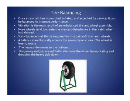
Tire balancing this is also a normal thing as we do in other automobiles also, once an aircraft tire is mounted, inflated and accepted for service it can be balanced to improve performance, vibration is the main result of an imbalanced tire and wheel assembly.
