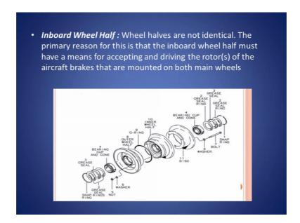
In this slide you can see the diagram, in the diagram you can see there is an outer wheel half, see this the outer wheel half the inner wheel half there are 2 wheel halves the outer wheel half the inner wheel half.
