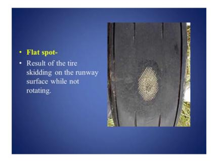
Now, flat spot this is the result of the tire skidding on the runway surface while not rotating. So, you can see the wear here see this wear pattern, this is the result of a flat spot.
