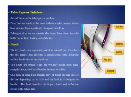
Tube type tires do not contain this inner liner since the tube holds the air from leaking out of the tire.
