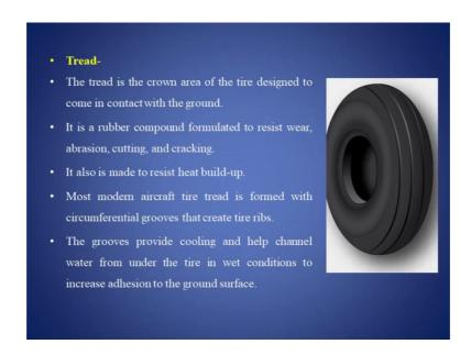
Tread, what is Tread? Tread is the crown area of the tire designed to come in contact with the ground, it is a rubber compound formulated to resist wear abrasion, cutting and cracking. It also is made to resist heat buildup most modern aircraft tires tread is formed with circumferential grooves that create tire ribs. So, in the diagram you can see these are circumferential ribs, you can see circumferential ribs in the diagram, you can see the grooves and these create the tire ribs.
