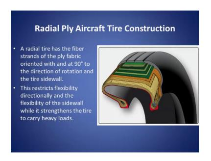
Now, radial ply aircraft tire or radial tire has the fiber strands of the ply fabric oriented with and at 90 degrees to the direction of rotation and the tire sidewall. So, this is the fabric orientation is 90 degrees to the direction of rotation and the tire side wall, this restricts flexibility directionally and the flexibility of the sidewall while it strengthens the tire to carry heavy loads.
