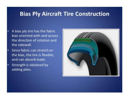
A bias ply tire has the fabric bias oriented with and across the direction of rotation and the sidewall.
