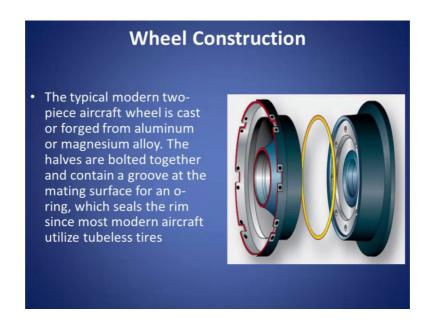
So, you can see in the diagram the wheel construction the wheel is in 2 halves.
