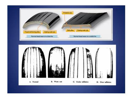
Now, in this diagram this is the normal condition, this tire is worn out; this is under inflation in case if you have been operating your tires under inflation condition. So, that wear will be of this pattern you can see the wear and incase your tire is has been operating in the over inflation condition, your wear will be of somewhat like this kind of thing.
