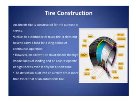
Coming to tire construction in the diagram you can see, a cross sectional view of a tire is given, an aircraft tire is constructed for the purpose it serves; unlike an automobile or truck tire it does not have to carry a load for a long period or of continuous operation.
