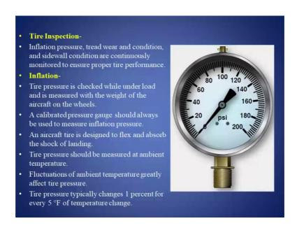
Now, what are the inspections on tire? Inflation pressure, tread wear and condition and sidewall condition are continuously monitored to ensure proper tire performance. So, during the time when the tire is used, almost in daily inspections inflation pressure is tested, tread wear and condition is checked, side wall condition is checked; these things are continuously monitored, so that proper tire performance can be achieved.
