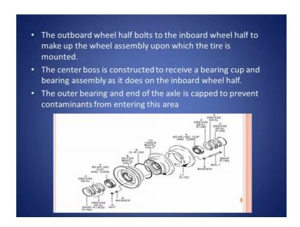
The outboard wheel half bolts to the inboard wheel half to make up the wheel assembly upon which the tire is mounted.
