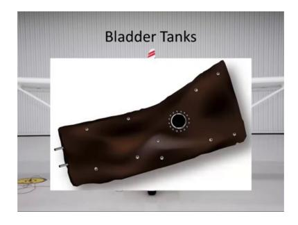
This is a sort of a bladder tank which is used in some of the aircrafts.
