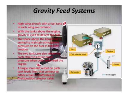
Now, the first type of fuel system is the gravity feed system. So, in this slide you can see the diagram this is the gravity feed system for the wings which are in the high position the fuel tanks, which are on the higher configuration.
