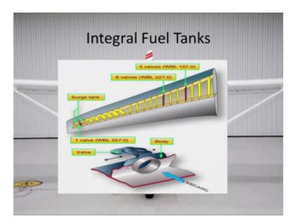
This is your integral fuel tank; in the integral fuel tank you identify a space in the wing and that space is used as a fuel tank.
