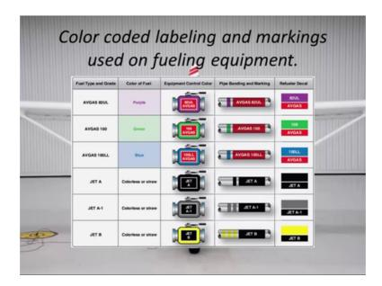
Now, in this diagram you can see the colour coded labelling and markings which is used on the fueling equipment. In the first column you see fuel type in red, second is colour of fuel, third is equipment control colour, fourth is pipe banding and marking and fifth is refueler decal.
