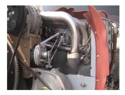
This is this is the hydraulic governor. You can see this is the hydraulic governor. This is attached to the linkage from the cockpit. And we check the governor for any leaks, for any damage, then we also move the control from the cockpit and check whether the control is free to move, whether there is no bindings. We will now move the control from the cockpit and show you how the control moves.
