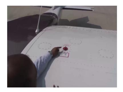
So, this is the top of the wing. This is the fuel tank cap, we remove this tank cap and the fuel is filled at this point. The maximum fuel tank capacity is 99, 92 gallons, US gallons. We have 2 fuel tanks, one in the left wing, one in the right wing. The fuel is filled from this point, this tank is opened, there are this; we need to be careful that this while locking that this has properly locked or not.
