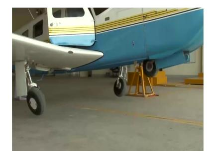
So, this is Piper Saratoga aircraft. You can see the landing gear of Piper Saratoga aircraft which is a retractable landing gear. Now you will see the retraction check. The retraction and extension check of Piper Saratoga aircraft. Layer up, you have seen that the landing gear, all 3 landing gears both main landing gears and nose landing gear have retracted. They are now up, we will now see how the landing gears are coming down, down you can see the grad gradual movement of the landing gears.
