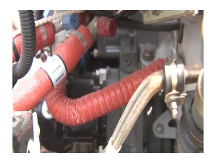
This is black component, this is magneto. There are 2 magnetos; one on the right side, one on the left side. So, in this air craft has got slick magnetos slick is the manufacturer.
