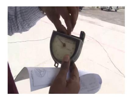
The cable tens the a block is fitted here and this is fixed on the cable and the tens and the tension recorded on this cable tensiometer. So, this is a very important check depending on the temperature on which you are operating and the cable size you get your cable tension get you prescribed. Tension limit by the manufacturer the your cable tension should be within that range. This tensiometer should also be periodically calibrated.
