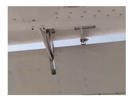
This is the control rod, this is the linkage points. During our inspection, we need to see that this rods they are there is no damage they are securely attached.
