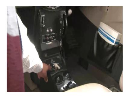
This is your fuel tank selection inside the cockpit. From here you can see you can select the fuel tank. At the movement this is your of position, this is your both position; that means, you can supply fuels simultaneously from both the tanks. You can either select the lack tank. This is your left tank selection.
