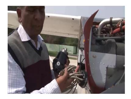
Then another critical component of the ignition system is the magneto. This is the magneto you can see this is the magneto. We have 2 magnetos. They are 6 6 3 5 1 auto magnetos installed on this engine. This is your distributor block, the distributor block and the ignition harness. This is the ignition harness. This distributor block the spark the spa the electrical sparks are generated in this electrical energy is generated in this magneto.
