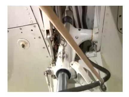
So, we are now on the Piper Saratoga aircraft which has a retractable landing gear. You can see the right main landing gear of Piper Saratoga aircraft.
