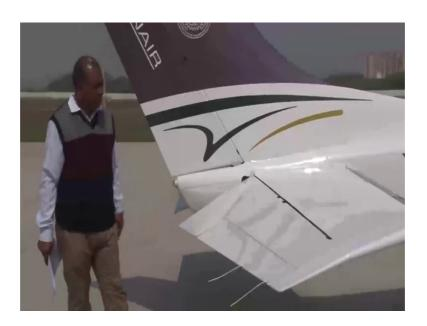
Another important control, this is the alleviator. The alleviator needs to be inspected as we have checked the alarms and the flaps. There should not be binding in the movement of control surface.
