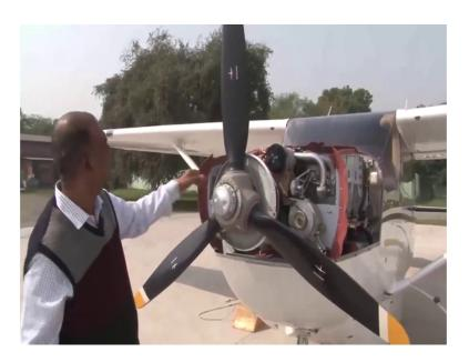
Then we come to the hub. This is the hub of the propeller. You can see the 3 blades attached; 1, 2 and 3. We will check the hub for cracks. The entire area of the hub is to be checked for cracks, any leakage, grease leakage.
