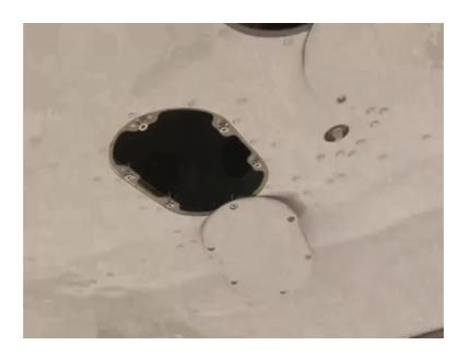
The once you have opened the inspection panels, you will check the internal structure also here you can see this is the rib. Similarly, you have the ribs all over. You check the ribs, there should not be any cracks, the internal skin there should not be any cracks and there should not be any deformation.
