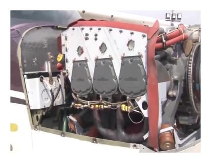
You can see the third one. This is the third mount and another mount on the other side. So, 4 mounts in all where your engine is mounted. As I have told that, this is the 6 cylinder engine, you can see 3 cylinders; 1, 2, 3 and 3 cylinders on the other side.
