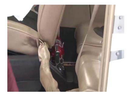
So, after the engine part, we will come inside the cockpit. These are the seats. The seats are to be inspected that they are serviceable and are installed correctly. Then, the seat movement on the rails the seat moves smoothly on the rails moves smoothly the the seats stops, the stops are here, the stops are here these stops are intact and the rails on which the seats are moving these are the rails, you can see here these are the rails.
