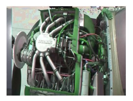
So, you can see the top view of the engine. This is your fuel air control unit. Fuel air control unit, then this is your air filter here. This is the air filter. These are the 3 cylinders here; 3 cylinders and 3 cylinders on the opposite side. These are the 3 cylinders. You can see the metal lines. These metal lines, these are the fuel lines. 3 spark plugs, these are the spark plugs. Then this is your induction manifold, your induction air going inside the cylinders.
