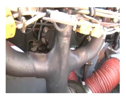
So, coming to the oil system of this engine, this is a wet slump lubrication system. You can see this is the crank case, this is the crank case, this is the place where the oil finally settles down; oil is there and this location this point this is the opening point, we in order to drain the oil from the system, we need to open this point, this is wire locked at the movement you can see after tightening it, we need to wire lock. So, remove.
