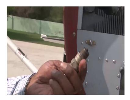
This spark plug is needs to be removed, cleaned and then installed back.
