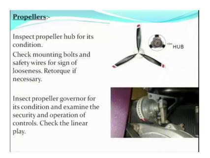
Propellers you inspect the propeller hub for its condition the spinner has been removed and inside is the hub we check the hub for condition we check the propeller mounting bolts and safety wires for sign of looseness and are re torque if necessary.
