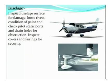
Then comes your fuselage inspect the fuselage surface for damage loose rivets condition of paint and check pitot static ports and drain holes for obstruction inspect covers and fairings for security as part of the hundred hours inspection the complete fuselage surface the fuselage skin has to be checked for any damage loose rivets the condition of paint has to be checked all over the fuselage.
