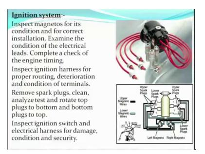
Coming to the ignition system inspect magnetos for its condition and for correct installation. Now you can see in the figure these are your magnetos we inspect the magnetos for condition and correct installation examine the condition of the electrical leads the electrical leads which are coming out of the magnetos.
