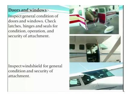
Doors and windows inspect the general condition of doors and windows check latches hinges and seals for condition operation and security of attachment. So, the doors and windows are to be inspected for condition operation all the locking mechanism all the latches the hinges are to be inspected for condition for security of attachment the door attachment points.
