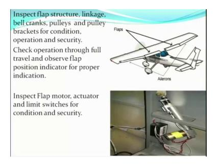
The flap structures the linkages bell cranks pulleys pulley brackets are checked for condition operation and security as part of the flight controls the flap system is also checked from the complete flap structure.
