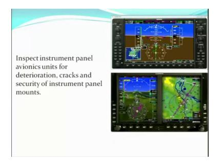
The instrument panels avionics units are inspected for deterioration cracks and security of instrument panel mounts. So, in the cockpit the instrument panels the avionics units are checked for deterioration cracks and security of the instrument panel mounts the fuselage.
