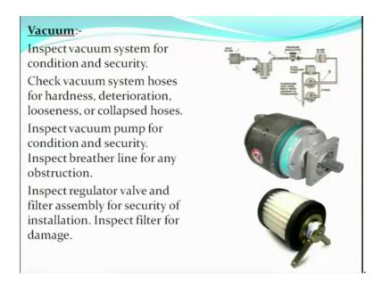
Next comes your vacuum system inspect vacuum system for condition and security this is in the diagram you can see this is a vacuum system here this is your drier vacuum
