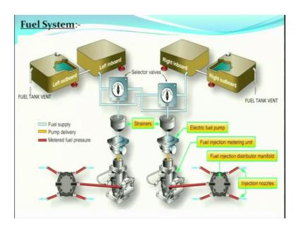
So, next is the fuel system you can see in the figure. This is the basic fuel system diagram shown the from the fuel tanks the fuel is coming to the filters, then to the fuel pump from the fuel pump, it is coming to the fuel air control unit or the metering unit from the fuel metering unit, it is going to the distribution manifold and then to the injector nozzles. So, this is just to brush up the fuel system.
