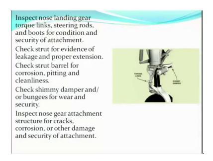
The axles here they also need to be examined for condition and security coming to the nose landing gear the nose landing gear these are the torque links this is your shimmy damper this is your nose gear strut we need to check the landing gear torque links these torque links the attachment points.
