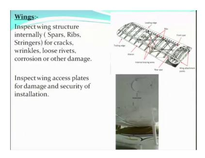
In the wings, the wings structure is inspected internally you have you can see the wings structure in the diagram there are spars you can see this is your front spar this is your real spar various ribs in the wing. So, we inspect the internal structure we inspect the spars the ribs different stringers for cracks wrinkles loose rivets corrosion or other damage.
