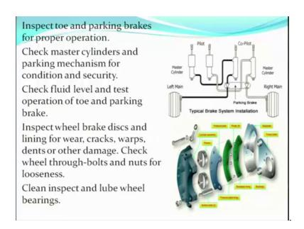
And parking break for proper operation now a part from the inspection on the landing gear the break part the breaks are also to be inspected the main breaks and the barking breaks are to be inspected for proper operation check master cylinder and parking mechanism for condition and security these are your master cylinders this is your break system of a typical aircraft these are your master cylinder which are there inside the cabin.
