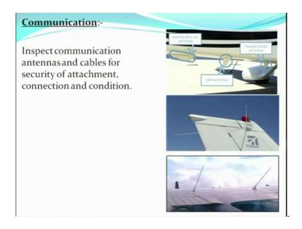
In the communication we inspect the communication antennas there are various antennas installed on the aircraft there is a marker beacon antenna dme antenna transponder antenna elt antennas navcom antennas various antennas are installed as part of the communication and navigation system the all the antennas and cables are checked for security of attachment connections and conditions.
