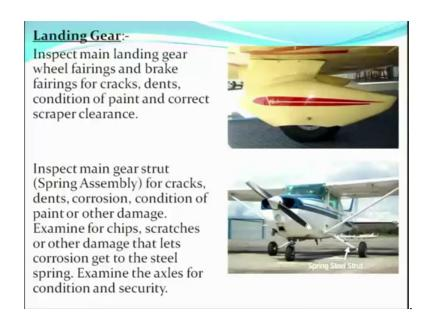
Then comes your landing gear inspect main landing gear wheel fairings and brake fairings for cracks. So, these are the fairings you can see these are the fairings on the wheels you need to inspect your main landing gear wheel fairings and a [bake/brake] brake fairings for cracks dents condition of paint and correct scraper clearance inspect main gear strut this is your strut assembly this is your spring steel strut inspect main gear strut for cracks.
