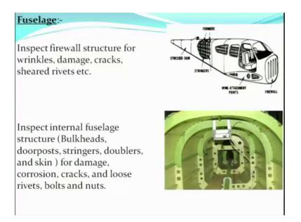
The fuselage the fire wall structure this is your fire wall in front of the fire wall is the engine installed this fire wall structure is checked for wrinkles damages cracks sheared rivets etcetera.
