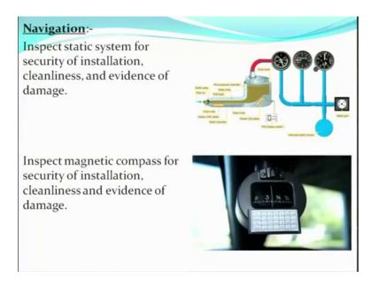
Now, coming to navigation inspect static system for security of installation cleanliness and evidence of damage. So, the complete pitot and static system this is the pitot tube the pitot tube is inspected the all the lines are inspected all the drain points are inspected the static ports are inspected for cleanliness evidence of damage for security of installation there is a pitot static leak check which is to be carried out.
