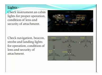
Next comes your lights check instrument an cabin lights for proper operation condition of lens and security of attachments check navigation beacon strobe and landing lights for operation condition of lens and security of attachment. So, in the hundred hours inspection we are inspecting all the lights in the cabin light outside the cabin light all navigation beacon strobe landing lights all lights are inspected for operation condition of lens and security of attachment.
