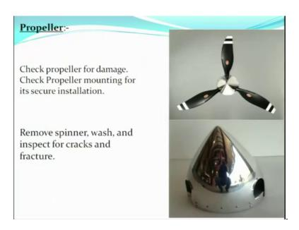
Then your propeller the propeller is to be inspected for any damage the propeller mounting is to be checked for secure installation.
