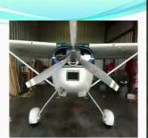
Then the propeller and the spinner, inspect the propeller blades for general condition and damage, especially near the tips leading and trailing edges, check installation for security.
