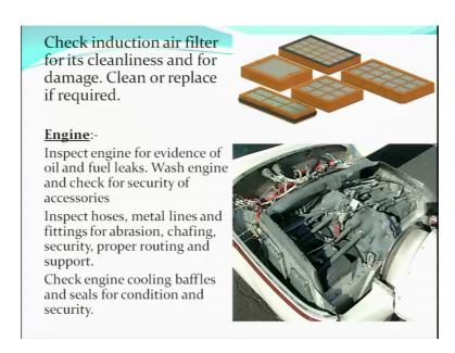
Check induction air filters for it is cleanliness, and for damage, clean or replace if required. The induction air filter is to be inspected for cleanliness and damage, and we need to clean or replace as required. So, in the 50 hours inspection, we are also cleaning the induction air filter, we may be required to replace it also. So, it is part of the 50 hours inspection.
