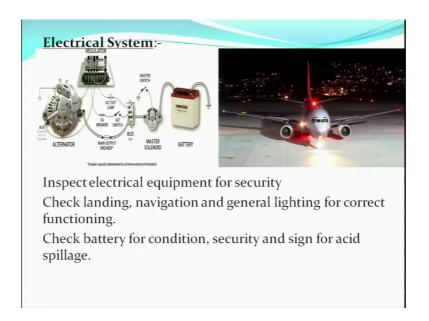
Coming to electrical system, inspect electrical equipment's for security, check landing navigation and general lightings for correct functioning, we also check the different lights, the landing lights, the navigation lights, and the general lights for proper operation, for proper functioning, check battery for condition security, and sign for acid spillage, we also check the batteries for condition, security and any spillage of the electrolyte.
