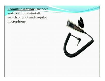
In the communication, we need to inspect and clean push to talk switch, this is this is the switch which is pushed while we talk, and the pilot communicates with the control tower, he use this push to talk switch, and this is inspected and cleaned during the 100 hours inspection.
