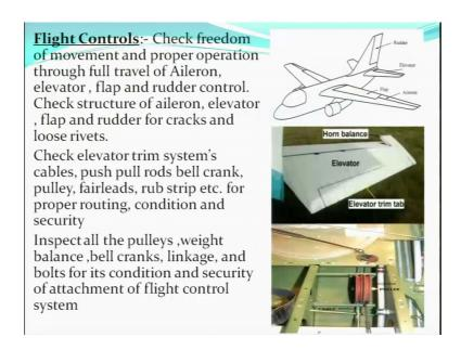
After this we come to the flight controls, check freedom of movement and proper operation through full travel of aileron, elevator, flap, and rudder control. So, all the flight controls ailerons, elevators, flaps, rudders, they need to be checked for proper operation through their full travel.
