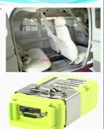
Then your equipment's and furnishings, inspect seats, seat tracks, rails stops restraint system for serviceability, security of installation, condition and for any damage.
