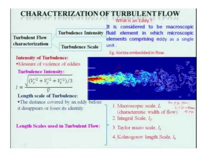
So, if you look at turbulent flow can be characterized by 2 quantities; one is turbulent intensity right and another is the turbulent scale right.
