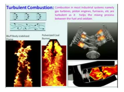
The laminar flow means the flow will be layer by layer. If you look at this is being shown here in this case is a flow through a pipe right is a layer by layer. That means, there would not be any mixing across the things, but where as in the turbulent right the flow will be not layer by layer it will be intermingling with each other right are you getting.
