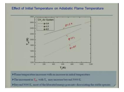
So, now look at this effect of initial temperature of adiabatic I am just elaborating little bit more further, that you can see that this are the corresponding to, what you call this is phi is equal to 1, and this is phi is equal to 0.5 and this is phi is equal to 1.5. And it goes on increasing with the temperature right.
