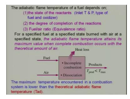
Now, to summarize about this adiabatic flame temperature; as we already know that adiabatic flame temperature of fuel depends on what equivalence ratio or the fuel air mixture. It will be depend on the initial pressure, it will be dependent on the initial temperature and also the type of fuel and oxidizer. It will be also depend of degree of completion of reactions; that means, extent of reaction is going on like whether it is
