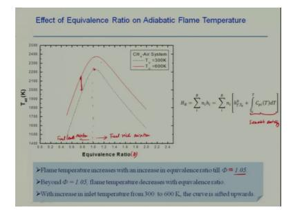
So, what I have taken here? This is methane air system and this is your peak value right, this is your 1. Is it peak for 300 Kelvin? This graph is for 300 Kelvin can black one, this adiabatic temperature here and this is equivalence ratio, this is phi. Is it peak here? No, peak is somewhere here right, peak is here this values.
