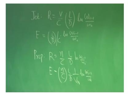
We are using that is precisely what is the engine being used if it is jet driven engine then we have seen R can be expressed as V by C, L by D to Ln W i minus 1 by W i, and for endurance it is L by D divided by C into Ln W i minus 1 by W i.
