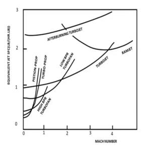
There and for different combination of engine different type of airplane a type of Mach number you are flying you can pick the value of C t based on historical data.
