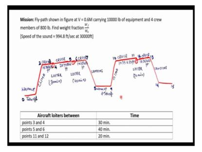
We have to calculate weight fraction Wf by W naught and for this calculation the speed of sound is 994.8 feet per second. As soon in the figure this is your mission profile aircraft loiter between point 3 and 4 for 30 minutes and point 5 and 6 for 40 minutes and point 11and 12 for 20 minutes. So, same problem only mission profile has been changed in this example.
