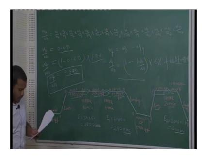
So, w f by w naught is one by w 14 by w naught into 6 percent fuel trapped. So, find the value of w 14 by w naught. So, w 14 by w naught is equal to w 1 by w naught into w 2 by w 1 into, w 3 by w 2, into w 4 by w 3, into w 5 by w 4, w 6 by w 5, w 7 by w 6.
