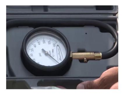
So, this is a tire pressure gauge we call it a TPG, it is properly calibrated we need to have a calibration tag, this calibration also has got a validity. Before using this instrument we need to ensure that your instrument is properly calibrated it is within the specified date limit, and then we need to measure the tire pressure. Please see the tire pressure and we will just show you how we measure the tire pressure.
