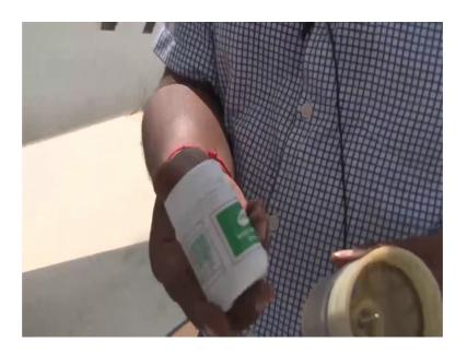
So, you can see this is a paste water finding paste, which we use to ensure that our sample or fuel sample or fuel in the aircraft tank is free of moisture.
