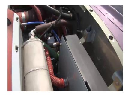
Here you can see the oil cooler; the oil cooler you need to ensure that your all cooler locking is in place, there are no leaks in the oil filter, that is it this is the oil cooler then you have the magnetos here.
