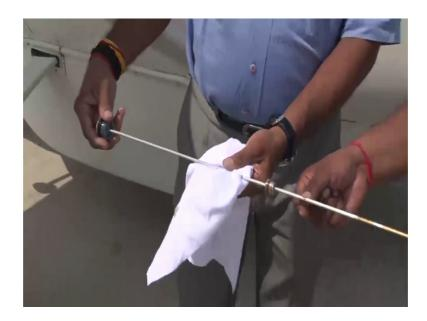
We will open this panel we need to see you can see the oil dipstick here, the oil tank cap. We will open this oil tank cap and ensure that the oil quantity is sufficient, you can see this is the oil dipstick, you can see the oil we will wash we will clean this lipstick with a
