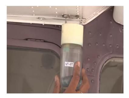
That the fuel is almost free of dirt there are no sediments and the fuel is safe for use this is a forward fuel drainage point this is the gascolator point we this is the lowest point in the fuel system. So, we want to take the fuel sample from the lowest point also to ensure
