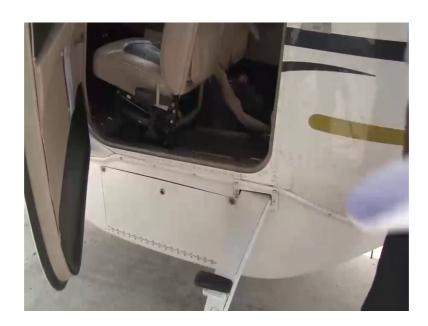
We this is the main undercarriage the main landing gear, we need to inspect the main landing gear for its cleanliness and condition, we need to watch do a visual inspection whether all the things are in place whether there is no crack. The main and nose wheel tires for creep marks general condition and correct inflation, you can see this is the main wheel.
