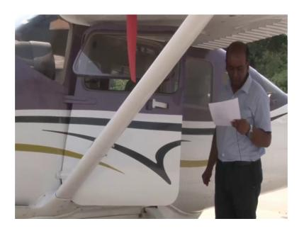
Going into the cockpit, we check for the general cleanliness and the general condition check seats and cushions for condition and security.
