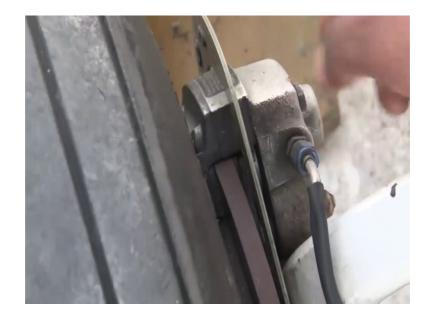
You can see the brake system here the brake unit, we need to watch we need to see that there are no leaks in the brake unit, there are the brake liner is there the brake liner has not worn off, and there are no leaks and no damage in the brake unit.
