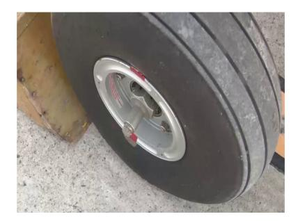
We need to see that the there are no cuts, no damage in the tire the required creep marks are in place, they require locking this split pin this is properly there, we need to inspect the main wheel. Similarly this is the left wheel similarly you need to inspect for the right wheel and the nose wheel; the brake system for leakage of fluid joints and for satisfactory operation.
