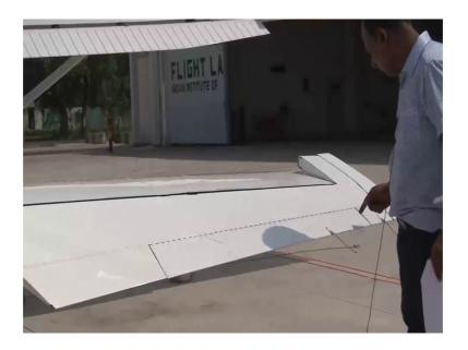
Coming to the trim tab check the hinge whether the hinges are in place the skin panel is there is no sharing of the rivets and the surfaces are neat and clean. These are the static discharge wicks you need to see these static discharge wicks, they have not worn out they are in place, the static discharge you can see they are all over all over the tail plane. So, you need to watch these static discharge weeks 2.
