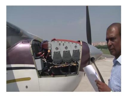
You can see the engine now this aircraft cessna 206 has got a 6 cylinder lycoming engine lycoming io 540 engine. Now coming to the engine this is the right side of the engine, three cylinders we see whether all the screws they are in place there are no leaks there are no leaks.
