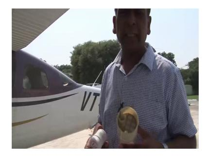
So, now, coming to fuel system, we need to take a sample of the fuel ensure that the fuel there are no sediments in the fuel, there is no dirt in the fuel sample, the fuel sample is free of water moisture.
