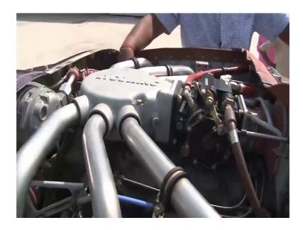
So, now, you can see the engine from the top you need to ensure that your cylinder fins, these are the cylinder fins you can see these are the cylinder fins, you need to see that there is no breakage there is no damage in the cylinder fins.
