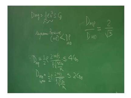
This will be will be equal to 2 by root 3. You see how it is happening I have miss some point here. So, drag minimum power will be half rho V square into S into C D. How much was C D for minimum power for the minimum power C D was 4 C D naught. We have shown that severally here I missed S into 2 C D naught right. Because we have seen C D for minimum power is 4 C D naught and C D for minimum drag is 2 C D naught we just we have shown that right.
