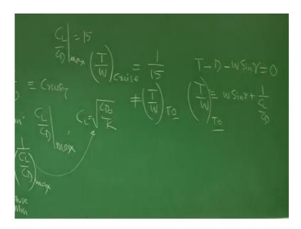
We have seen that if I write T minus D minus W sin gamma, and if I am to takeoff without any acceleration that is steady climbs small climb I am doing, then T by W is roughly equal to W sin gamma plus 1 by C L by C D, we have shown the roughly this is approximately.
