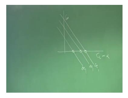
And before that it has summarized what we are talking, but I can trim the aero plane at different C l or alpha and for different delta e different delta requirement will be there, if you want to trim at here or here and the question is, is my elevator enough powerful to generate or to trim the aero plane? That is the question right.
