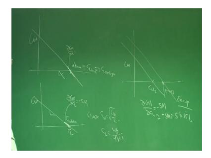
In that connection we realize that if I plot Cm versus alpha, then if this is my alpha trim, it is which corresponds to Cl trim which say Ci design. I can visualize like this and this slope at trim will say d Cm by d alpha. I can visualize it through Cm versus Cl, where this is directly Cl design and the slope here at the equilibrium is minus static margin.
