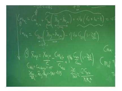
If we recall the expression for neutral point, neutral point bar was x ac wing by c minus Cm alpha fuselage by Cl alpha wing plus eta v h Cl alpha tail by Cl alpha wing 1 minus d epsilon by d alpha, where d epsilon by d alpha is approximately C l alpha wing by pi aspect ratio of e.
