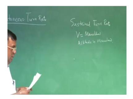
So, that is what is we talking about is instantaneous turn rates and it not take condition it should maintain the speed or altitude and you can understand in contrast instantaneous turn rate is sustained turn rate where the condition is that I am doing a turn same time the speed should be maintained V maintained as well as altitude is also maintained.
