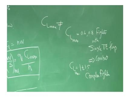
This is given by this, but please be careful this C L max is not as high as C L max when you talking about takeoff or landing right, but this value typically will be C L max for all practical purpose. It will fight 0.6 to 0.8 for fighter with single trilling edge flap during combat. This is important during combat; you never would like to use all these things during normal flight plus lot of penalty increase.
