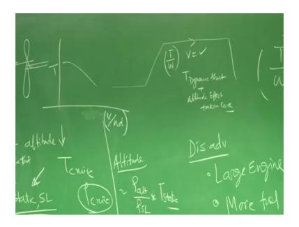
So, I need to know what is the dynamic thrust available during the operation that is if I am talking about cruise I will moving with some speed if I talk about T by W here the T should be the dynamic thrust dynamic thrust plus the altitude effect taken here right; this is extremely important.
