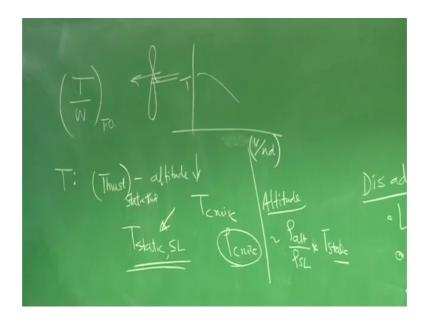
And if I write (Refer Time: 24:24) what here I must take if I talk about thrust. So, realize that thrust what you are talking about static thrust their availability with altitude will drop. So, without jet engine on a propeller driven engine I C driven we find as altitudes increases the density where they are air reduces.
