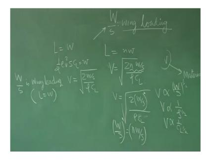
Ah v equal to 2 W by S by rho C L under root this is the speed required to maintain lift equal to weight at an altitude rho which is flying at a given C L.
