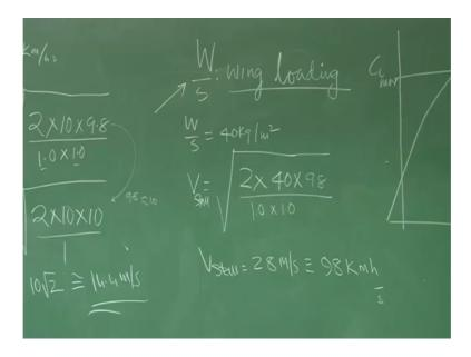
So, what do I am saying is W by S is 40 kg per meter square. So, we will be V stall will be 2 W by S is 40 again into 9.8 to convert a newton rho I have taken one and C L I have taken one please understand C L typically is 1.2 maximum you get for V stall all I need to take C L max, but we are taking it 1. And this also now comes out to how much.
