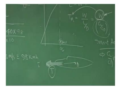
This or that what you require you require this is the airplane we require the thrust of the power should be capable enough to overcome the drag experience by it, as to maintain the speed which we are demanding.
