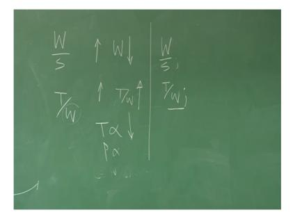
So, you are loosely talking about very loosely you are talking about, wing loading and thrust loading just to give you understanding introductions because you have to go in detail about those things in the design, but one thing you understand that as I am going higher and higher, the W will go on reducing do not forget that.
