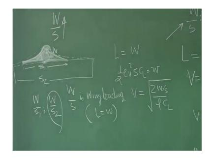
You could easily understand, if I go on increasing the wing loading meaning thereby what does it mean if I go on increasing, the wing loading; that means, I am relatively I am reducing the wing area.
