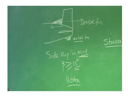
Now, this the dorsal fin; this is primarily required slip in side slip in mind. Suppose a airplane because of some reason has gone into high side slip; could be it has made an entry into spin, I see side slipping very fast and the moment the side slip angle, let us say this is more than 15 degrees and there is every possibilities of vertical fin may stall. A vertical fin stalls; rudder also will be ineffective; so you will not be able to control.
