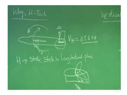
So, horizontal tail is extremely important from the static stability point of view and also it has to house elevator with horizontal tail; part of it can go down, can go up and it acts an elevator and the elevator effectiveness depends upon, the ratio between elevator area or the tail area S t and elevator area.
