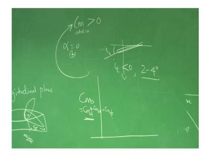
We try to give a setting angle to the horizontal tail i t; which is negative maybe order of 2 to 4 degrees; typical numbers. This is done to ensure that even the if alpha equal to 0, it has a force here and cg suppose is here it gives you a C m at alpha equal to 0 or C m naught greater than 0.
