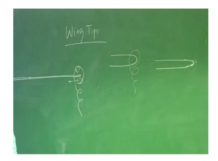
Another important part of wing; wing tips and you know what is; so, importance about wing tips we know that our aim is to ensure high L by D and one way to increase L by D is to reduce induce drag and induce drag phenomena is something here, but the vertices from here because of pressure this differences. So, if you want to reduce this induced drag somehow I should discourage the tendency of the flow from high pressure to lower pressure region.
