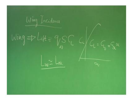
Now, next step is what we will be discussing and sharing what is there in that domain of aircraft. When you talk about wing, we also should talk about wing incidence. What do I mean by that? Fundamentally, wing is primarily to give lift and lift; we know this is dynamic pressure S into C L and C L is depending upon type of aerofoil you are using, so C L is; C L naught plus C L alpha into alpha.
