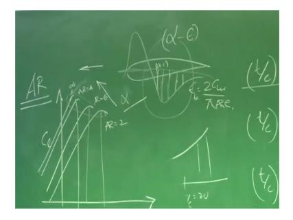
So, it will not stall it may stall a at our 17 degree. What do we say if aspect ratio is large the epsilon will be small, so it will have lesser stalling angle, but if aspect ratio is small epsilon will be large. So, the stall angle will increase and that is exactly happening as aspect ratio increasing the stall angle is decreasing right.
