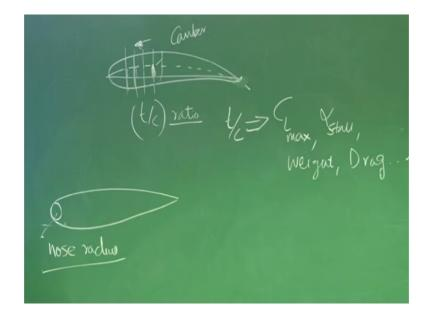
When we are talking about aerofoil so, I draw the aerofoil one words to say the camber line or the camber right and you know if I draw this curved line then draw perpendicular to the card and this distance is the camber. If it was symmetric the card and the cambered line would have been in same or coincident to say camber is 0.
