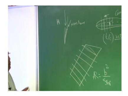
Aspect ratio of when you say this is band squared by the area of the wing, and sweep also you know of this is the aerofoil and flows like this, if I drag my aerofoil like this then there is a component which is M cos of sweep angle.
