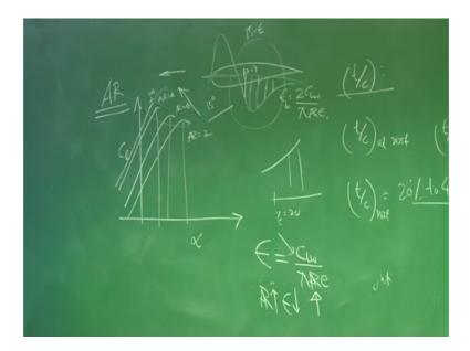
Since we are graduating from aerofoil to wing and that is aspect ratio right and if we recall our studies (Refer Time:39:06) performance goes, to find that this is aspect ratio some number I am giving it is a aspect ratio 6, this is aspect ratio 8 and close by it will be aspect ratio infinity.
